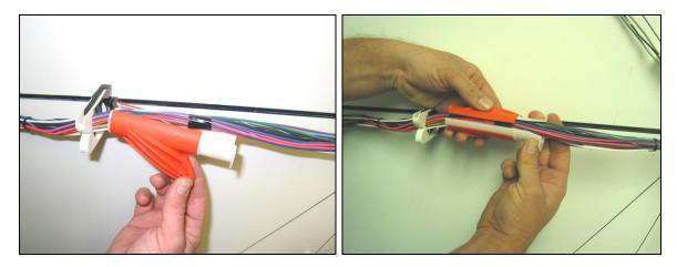
The wire is inserted into the tool. The tool is then closed around the wire
