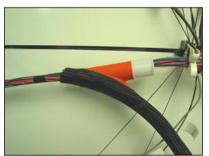
The "spreader" of the tool is then inserted into the ClassicBraid. With the tool inserted, pull the tool down the length of the ClassicBraid. This will insert the harness into the braid as it is pulled.
