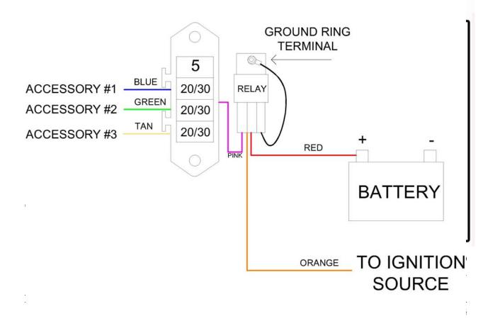
E: POPULATE THE FUSE BLOCK WITH THE APPROPRIATELY RATED FUSE FOR EACH CIRCUIT. KEEP IN MIND THE RELAY IS DESIGNED TO HANDLE 70 AMPS OF CONTINUOUS CURRENT. DO NOT ATTEMPT TO DRAW MORE THAN 70 AMPS OF CURRENT THROUGH THIS CIRKIT BOSS KIT. DOING SO WILL CAUSE PREMATURE FAILURE OF THE RELAY.
