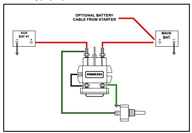
Solenoid draw is 2.5 AMP while engaged. If left engaged, with vehicle not running, it will drain the battery!
