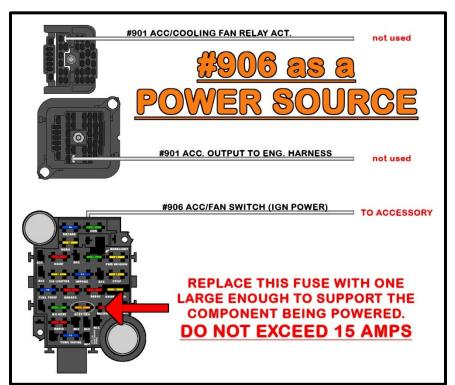
Wire **#906** can be used to power an accessory inside vehicle. This could be anything from additional gauges, a USB port, a wideband O2 controller, rear-mounted fuel pump relay, etc. If powering an accessory, make sure to replace the 5-amp fuse in the fuse block on the circuit labeled "ELECTRIC FAN".
