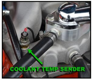
to, as seen in the photo above. Ring terminals and insulated spade terminals have been provided. Your factory notched connector will need to be re-used if your sender has a round disk on top.
