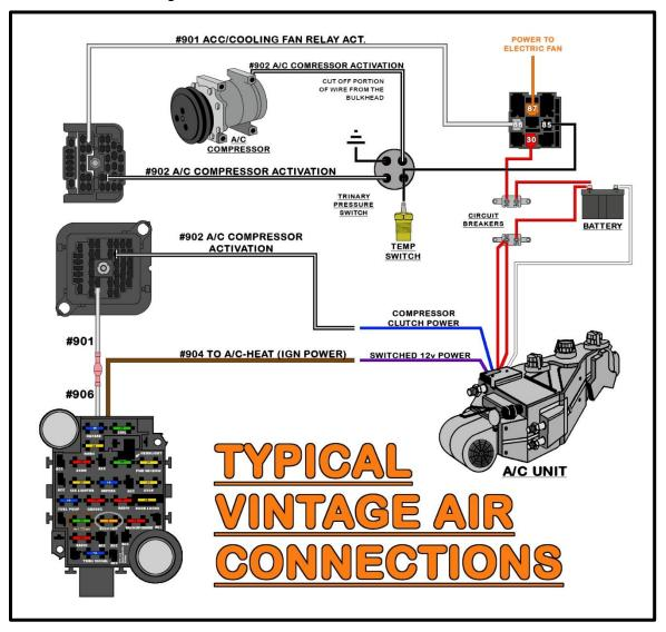
Your aftermarket system should come with all the wiring needed for proper operation. This wiring will need to be connected to power sources provided by the battery and the Painless harness. The diagrams are labeled as "Vintage Air" and the wire colors are those used by Vintage Air. These same connections hold true for any aftermarket system, regardless of the manufacturer or the wire colors they use.
