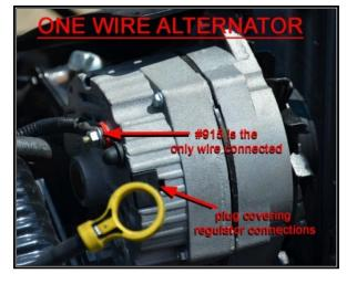
**POWER (BATTERY)**, this is the sense wire, it provides a battery power source, or voltage sense, that all voltage regulators require. This wire always has power and comes from the large battery supply splice in the harness. This wire will not be needed if you have a one wire alternator or a GM CS series alternator. See the various alternator illustrations on pages 54 – 65 and the *Charge/Battery Power Schematic* on page 51.
