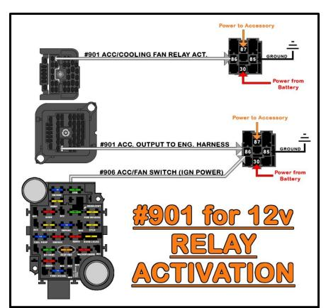
If you need to power an accessory in the car, but also need relay activation in the engine compartment, simply double the #901 and #906 wire together as shown here.
