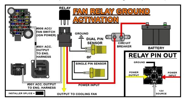
If A TOGGLE/ROCKER SWITCH IS BEING USED WITHOUT A RELAY, MAKE SURE THE AMPERAGE OF THE COMPONENT YOU ARE POWERING DOES NOT EXCEED THE CAPABILITIES OF THE SWITCH OR SWITCH FAILURE WILL OCCUR. IF YOU NEED A RELAY KIT PAINLESS OFFERS PART #'S 30128, 30128, & 30130.
