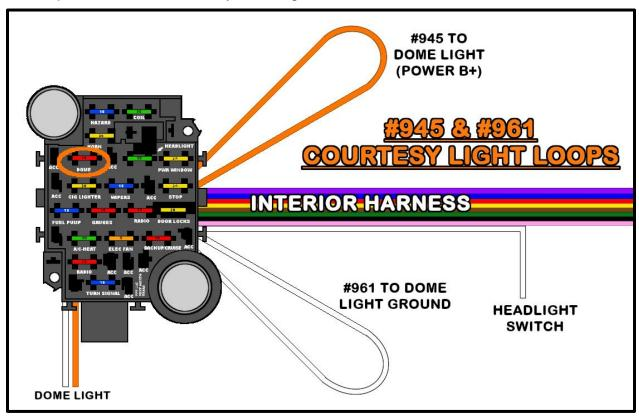
o If you do not want to wire in jamb switches or courtesy lights, the WHITE #961 wire in the Tail Section and the other end of the #961 wire in the Headlight Switch Section can the pulled taut in order to remove the loop from the harness. The same can be done with the ORANGE #945 wire in the Tail Section.
