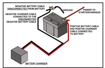
battery and make sure the other end of this cable is connected to the B+ side of the starter solenoid.
