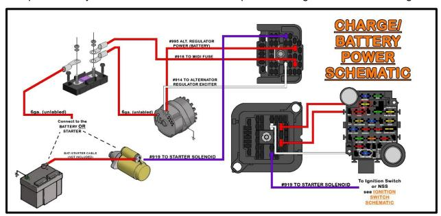
Locate the bag kit provided with the Painless harness kit labeled "ALTERNATOR." This bag kit contains the hardware needed to make the appropriate connections to the alternator as well as a covered inline fuse holder.
