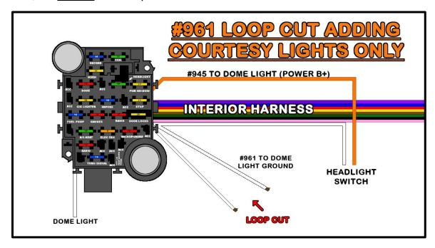
Create a splice or splices that will provide a wire to each courtesy light. This splice will
