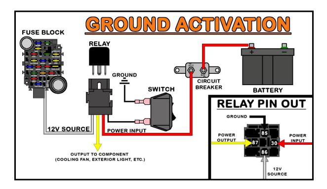
A ground activated relay is just the opposite of the 12-volt, activated relay; 12 volts (battery constant or switched) are supplied uninterrupted and the ground wire is switched. The Horn Relay pre-wired in the Painless harness is a Ground Activated Relay. Another example of this method is a thermostat operated fan relay. In this case, however, a thermostatic switch would replace the switch in the drawing above (see below).
