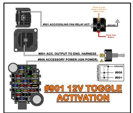
The diagram to the right depicts the most common way #906 and #901 will be used: #906 and #901 connected, with #901 in the engine compartment providing 12v to a fan relay. The relay is then ground activated using a temperature switch installed on the engine. offers **Painless** numerous Fan Relay Kits, part #30100 thru #30130.
