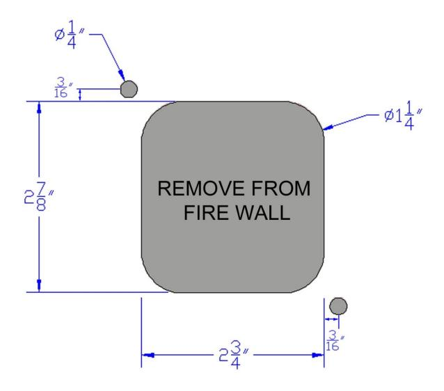
NOTE: This drawing MAY NOT be to scale, please double check your measurements with those on the drawing before any cutting or drilling.
