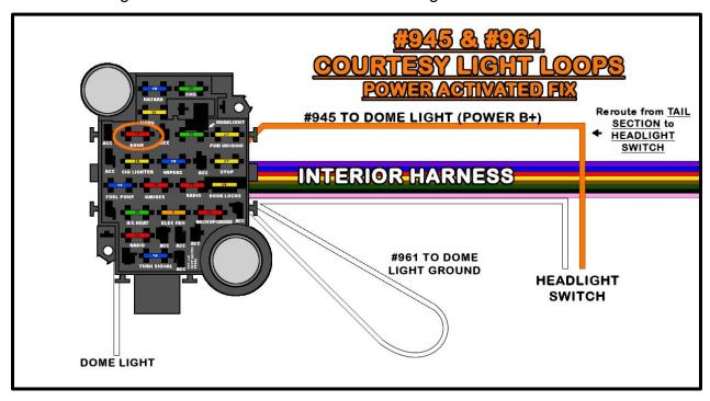
• If you also wish to add courtesy lights to under the dash, a center console, pillar lights, etc., the WHITE #961 loop will need to be cut.
