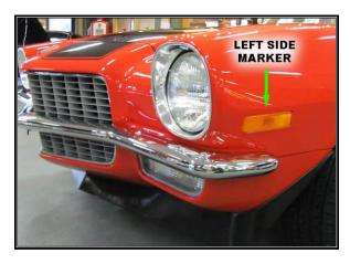
The park light feature is activated by a power source coming from the headlight switch. This light illuminates any time the headlight switch is in the "PARK" or "ON" position. The turn signal feature is provided by a power source coming from the turn signal switch.
