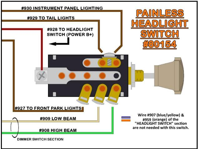
Painless offers several universal switches as well, and even one with hi-low beam dimmer functions. Use the following diagrams to connect to either of the universal headlight switches offered by Painless. Use the blue insulated ring terminals found in the parts kit to make these connections.
