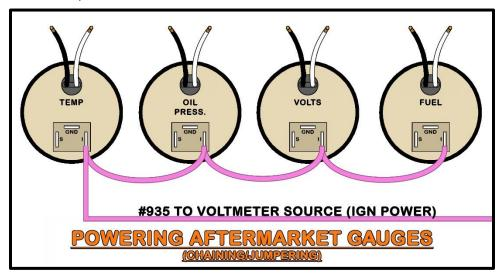
Grounds need to be supplied to the gauge lights and any ground tab on the gauges. The installer needs to run their own ground circuit for gauge connections. To make these ground connections you can splice from the installer provided ground wires to all the gauges or chain/jumper it all together. Both methods can be seen in the following two drawings:
