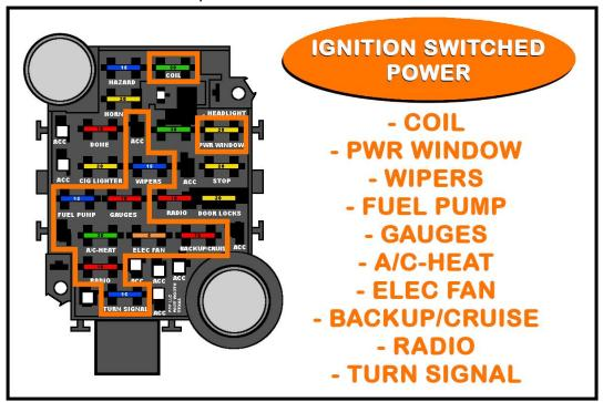
The drawing above shows all the switched ignition fuses. These fuses are powered by wires coming from the ignition switch (wires #931, #932, and #933) and receive power depending on what position the ignition switch is in. NONE OF THESE FUSES SHOULD HAVE POWER WHEN THE IGNITION IS IN THE OFF POSITION. The Ignition Switch Section beginning on page 93 of this manual will go into further detail about power supplied to these fuses.
