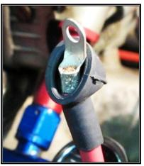
If your vehicle has an aftermarket, **ONE**WIRE ALTERNATOR, meaning it does not require a switched 12v source or regulator connections, or if the Painless or other aftermarket fuel injection harness you are using has an alternator connector, then this output wire is the only wire used in this section at the alternator.
