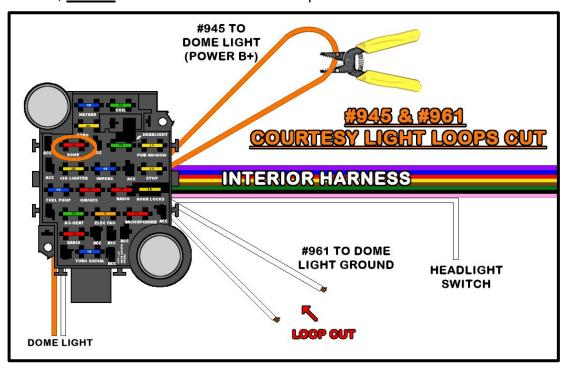
• The dome light connection in the <u>Tail Section</u> will typically connect in the trunk above the driver side rear wheel to a factory pigtail. This means the <u>ORANGE</u> #945 and the <u>WHITE</u> #961 wires will have a considerable amount of length removed. These pieces of wire cut from the <u>Tail Section</u> can be used for your jamb switch and courtesy light connections.
