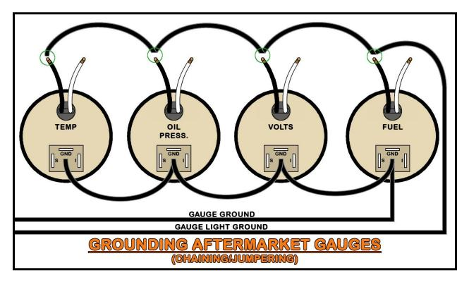
Gauge light power is supported by the **BROWN #930** wire. This wire connects to one of the leads for the gauge light or the gauge light tab found on gauges with LED backlighting. To make these connections you can splice from this **BROWN #930** wire to all the gauges or chain/jumper it all together.
