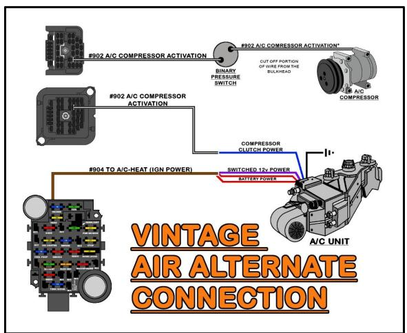
Locate the wire(s) from your A/C unit that are intended to be connected to the battery
