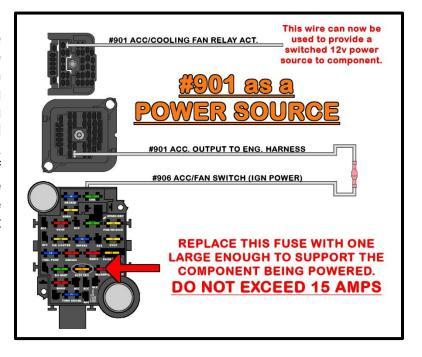
If a rocker or toggle switch is desired to control an accessory or accessory relay, #906 and #901 will need to be wired to the switch. A ground wire will be to be added for those using a switch with backlighting
