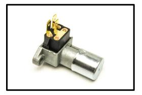
The connection point of these wires depends on the location of the dimmer switch. Most have a floor-mounted dimmer switch, although, those using a later model GM column may find the dimmer switch on the side of the column. Painless offers part #80150 for those needing a new floor-mounted dimmer switch.
