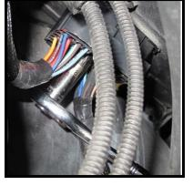
• Using a 3/8" **socket**, tighten the mounting thru-bolt on the engine bulkhead to the firewall connector. **DO NOT OVERTIGHTEN!** The bulkhead connector can/will crack and the threaded insert in the firewall bulkhead can strip or loosen the threaded insert in the fuse block mounted bulkhead connector.
