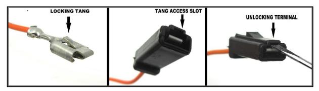
With this harness being universal, many of your factory connectors or factory service pigtails will need to be re-used. Factory terminals have been provided to allow re-using the connector without having to splice to existing wires. The removal process of wires into factory style connectors is as followed:
