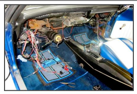
During the removal of the old, factory harness, avoid making any unnecessary cuts to any wires. The entire harness should be able to come out of the vehicle without any cutting at all unless someone has modified connections.
