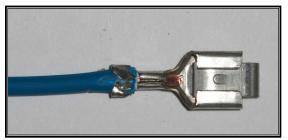
• Using the appropriate jaw on the crimpers, crimp Strap 1. The appropriate jaw depends on the wire gauge as well as the terminal stiffness. If you are unsure which jaw to use, you can always start with the biggest and work your way down until you get a tight crimp.
