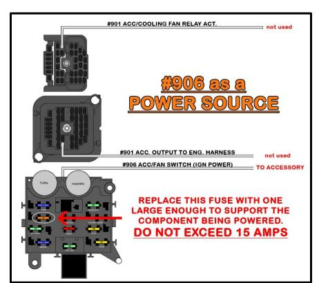
Wire #906 can be used to power an accessory inside the vehicle. This could be anything from additional gauges, a USB port, a wideband O2 controller, rear-mounted fuel pump relay, etc. If powering an accessory, make sure to replace the 5-amp fuse in the fuse block on the circuit labeled "ELECTRIC FAN".
