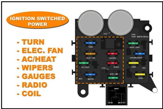
The drawing above shows all the switched ignition fuses. These fuses are powered by wires coming from the ignition switch (wires #931, #932, and #933) and receive power depending on what position the ignition switch is in. NONE OF THESE FUSES SHOULD HAVE POWER WHEN THE IGNITION IS IN THE OFF POSITION. The Ignition Switch Section beginning on page 92 of this manual will go into further detail about power supplied to these fuses.
