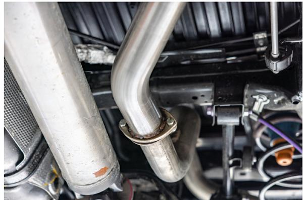
**Step 3:** Install new MagnaFlow Muffler by first sliding the outlet onto the OE System and then bolting the MagnaFlow flange to the OE flange using the OE fasteners.
