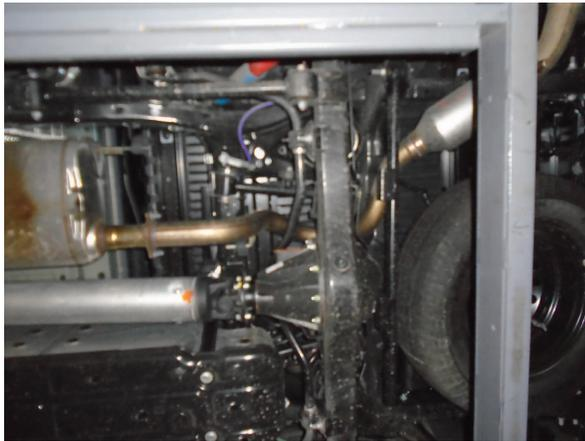
Remove the OE Muffler by loosening and removing the bolts at the outlet flange. Then disengage the hangers from the rubber insulators. Do not damage the rubber insulators or discard the fasteners as these will be used for the new MagnaFlow Muffler.
