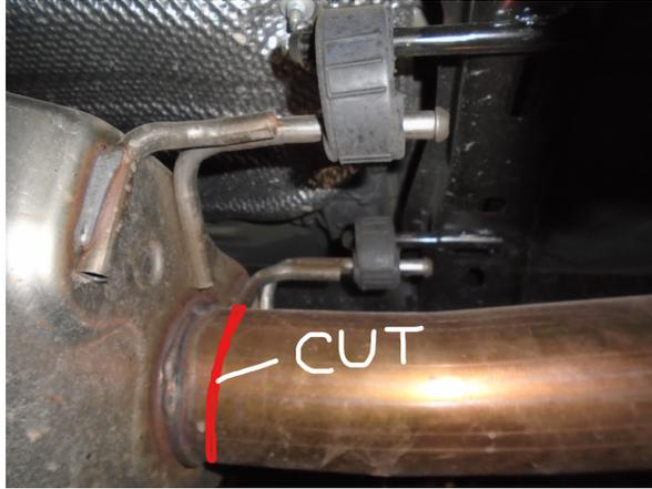
Begin removal of the OE muffler by marking cut point a 1/2" to the rear of OE Muffler as shown in photo below. Then cut the OE Exhaust at that cut point.
