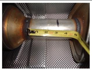
**Step 1:** To install the MagnaFlow exhaust the OE system must be cut. Measure 3.00" back from the catalytic converter weld, cut at this point and deburr pipe. Working front to rear disengage all welded hangers from the rubber insulators. The OEM exhaust system can now be removed in one piece. Be sure to retain the rubber hanger insulators as they will be needed to install your new MagnaFlow system.
