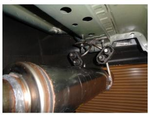
**Step 4:** Using the existing studs located on the factory frame rail mount the supplied Hanger Assembly with the supplied M8 lock nuts and washers.
