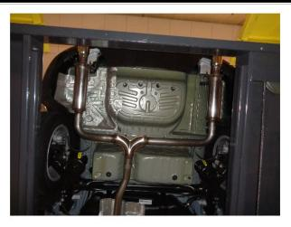
**Step 5:** Next **s**lip the P/S Muffler Assembly onto the Y-Pipe Assembly and loosely fasten with the supplied 2.25" Clamp. Using the supplied Rubber insulators attach the hangers. Fit the D/S Muffler Assembly in the same manner using the supplied clamp and OE rubber insulators.
