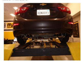
**Step 6:** Once a final position has been chosen for the new exhaust system, evenly tihgten all clamps from front to rear using the torque specifications on page one of these instructions. Inspect all fasteners after 25-50 miles for operation and re-tighten if necessary.
