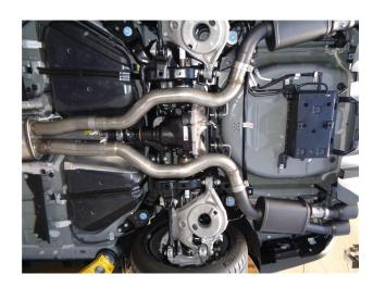
**Step 4.** Next attach the Mid Pipe Assemblies to the X-Pipe using the supplied 3.00" clamps and fitting the hangers into the rubber insulators.
