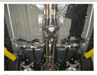
**Step 3.** Begin installation of the new system by loosely attaching the X-Pipe Assembly to the outlets using the OEM clamps. Leave all clamps loose until final adjustment.
