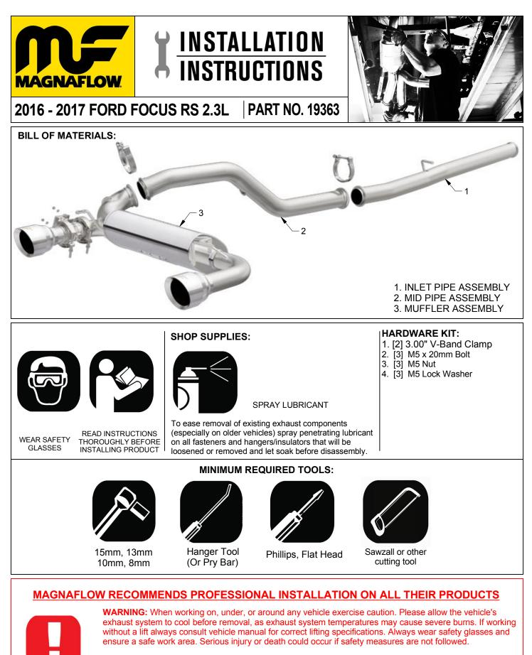
**ATTENTION:** Always install any supplied band or V-band clamps to the proper torque specifications of 40-45 ft-lbs for band clamps and 70 in-lbs for V-band clamps. Over tightening will result in the clamp breaking and will NOT be warranted by MagnaFlow.
