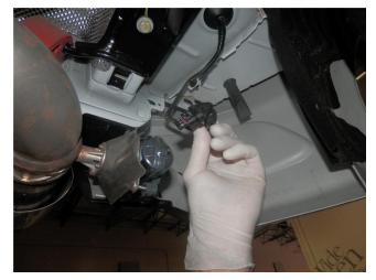
**Step 1.** Before removing the OEM exhaust you will first need to unplug the electrical connection on the exhaust valve control motor located on the OEM muffler assembly.
