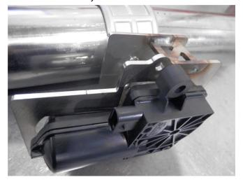
**Step 3.** You will need to cut the OEM system at the Over Axle point to remove it. Once the OEM system has been removed transfer the exhaust valve motor to the Magnaflow system using the supplied hardware (M5 fasteners). The alignment spring on the motor will need to be engaged into the keyway slot of the new valves.
