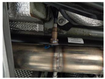
**Step 5.** When reattaching both O2 sensors to the Inlet Pipe Assembly take care as each sensor has a different thread pattern.
