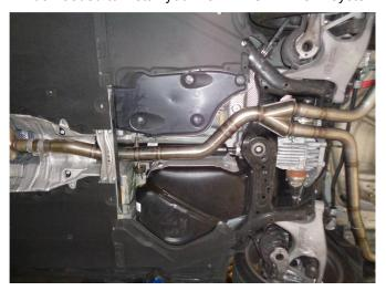
**Step 3.** Begin installation of the new system by slipping the inlet of the Inlet Pipe Assembly into the outlet clamp of the DPF assembly using the OEM hardware. Engage the welded hanger to the rubber insulator. All clamps should remain loose until final installation is complete.
