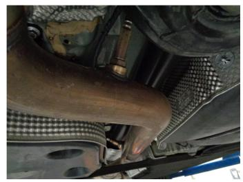
**Step 1.** To remove the OEM exhaust system first revomve the two O2 sensors attached to the inlet pipe.
