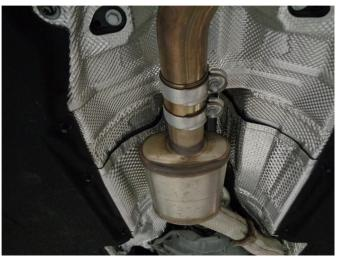
**Step 2.** Next, unbolt the clamp attaching the inlet pipe to the DPF. Working front to rear remove all welded hangers from the rubber insulators. The exhaust system may now be removed. Retain all mounting hardware as it will be needed to install your new MAGNAFLOW system.
