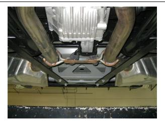
**Step 1.** Begin by removing the two rear chassis stiffeners by the muffler inlets. This will allow access to the exhaust system.
