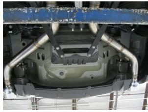
**Step 3.** Install the new system by attaching the Driver and Passenger Tailpipe Assemblies to the cut portion of the OEM system using the supplied 3.00" clamps. Leave clamps loose for final adjustment. Fit the hangers into the rubber insulators.
