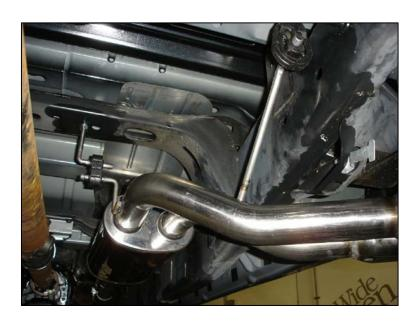
**Step 3:** With all components mounted loosely, adjust the system for overall aesthetics and clearance of frame & bodywork. (MAGNAFLOW recommends at least 1/2" of clearance between the exhaust system and any body panels to prevent heat-related body damage or fire.)
