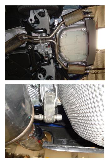
**Step 3.** Next, install the Mid Pipes to the Resonator Assembly using the supplied 2.25" clamps. Finish by attaching the Muffler Assemblies to the Mid Pipes using the supplied 2.25" clamps. Insert hangers into rubber insulators.
