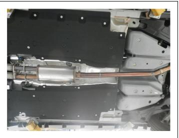
**Step 3.** Begin installing your new system by loosely attaching the inlet flange of the Resonator Assembly to the flex outlets using the OEM fasteners (leave all clamps and fasteners loose until final position is chosen). Next, install the Mid Pipe to the Resonator Assembly using a supplied 2.50" clamp.
