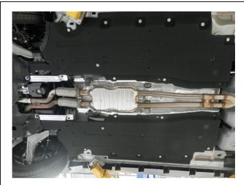
**Step 1.** Begin removing the OEM exhaust system by unbolting the flange at the flex assembly outlets. Retain the mounting hardware and rubber insulators as they will be needed to install your new system.
