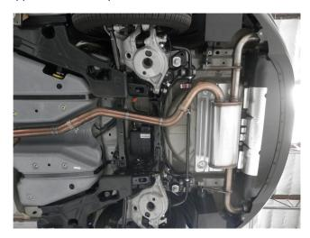
**Step 4.** Install the Connecting Pipe to the Mid Pipe using a supplied 2.50" clamp. Finish by inserting the muffler tips into the openings in the rear valance then attaching the Muffler Assembly to the Connecting Pipe using a supplied 2.50" clamp and inserting the hangers into the rubber insulators.
