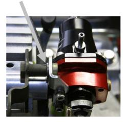
9. In some installations it may be necessary to relocate the return line mounting clamp. Using the enclosed cushioned line clamp as a pattern, mark the OEM line bracket and drill a hole using a #18 drill bit (.170 Diameter).
