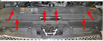
16. Using a 10mm socket, remove the six (6) top support bolts securing the fascia.
