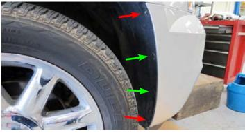
18. Using a 10mm socket, remove four (4) bolts from the bumper/fender support brackets. Two (2) from the driver side and two (2) from the passenger side.
