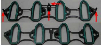
71. Install the modified intake manifold gaskets onto the supercharger manifold using the installed bushings as guides. Proceed to Step 73.
