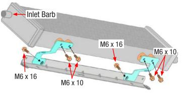
88. Secure the upper LTR bracket to the LTR with two (2) 1" spacers and two (2) M6 x 35mm bolts from the SUV hardware bag. Now secure the LTR to the hood latch location using two (2) M6 x 16 bolts along with two (2) M6 nuts. Proceed to Step 91.
