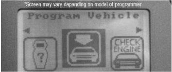
4. Use the directional pad to highlight the Pre-programmed Tune option and press the Select button.
