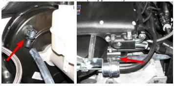
106. Install the driver side PCV hose by sliding it onto the rear barb located on the driver side valve cover. Then install it on the center barb located on the manifold nose. Be sure to route the hose between the coil bracket and intercooler hose.
