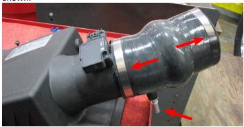
121. Reinstall the top cover by slipping the silicone elbow onto the throttle body first. Then secure the top cover using a Torx T25 and the factory airbox screws. Re-align elbow for best fitment and tighten both worm clamps.
