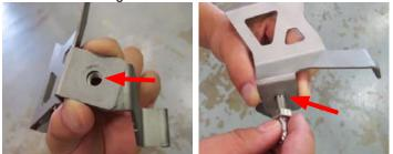
130. Position the hood dampener bracket assembly under the rain guard and align with the hole on the OE hood dampener bracket. Adjust the bracket so that it sits flush on the OE bracket and the firewall. Mark the location of the rear mounting hole with a marker.
