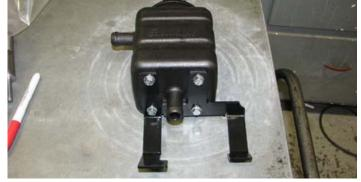
99. Connect the Manifold to Recovery Tank hose to the recovery tank's inlet barb using one (1) 3/4" hose clamp. Connect the Tank to Water Pump hose to the tank's outlet barb and secure with one (1) 3/4" hose clamp. Route Tank to Water Pump hose down towards the left front of the vehicle. Then install the tank onto the two (2) front passenger side coil pack studs with two (2) M6 nuts from Bag #2.
