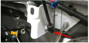
128. Remove the factory clip securing the rain guard.
