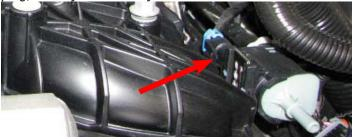
28. Remove the brake booster hose from the check valve. *NOTE: Retain the check valve for re-use.*
