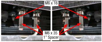
91. Secure both ambient air temp sensors onto the lower LTR brackets as shown (one to each bracket).
