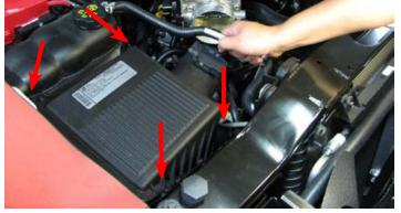
119. Replace the factory air filter with the supplied Green reusable air filter.
