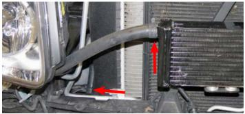
93. Route the LTR to Manifold Hose along the bottom of the lower radiator fan shroud and install onto the lower passenger side manifold inlet barb. Using four (4) wire ties, secure the hose to the lower radiator shroud.
