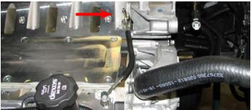
68. Remove the rear engine support brace attached to the rear of the driver side cylinder head using a 15mm socket.
