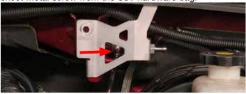
133. Using two (2) 13mm wrenches, secure the hood prop bracket to the OE bracket using the M8 bolt and M8 nut from the SUV hardware bag.
