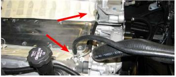
66. Using a razor blade or equivalent, remove the rubber guard on the factory coolant crossover and install it onto the supplied coolant crossover.
