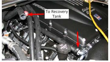
97. Then route the hose behind the manifold and install it onto the upper driver side manifold outlet barb.
