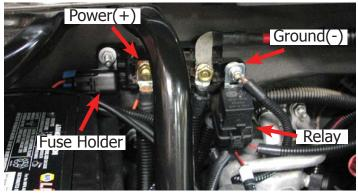
**NOTE:** Step 124 is for vehicles with battery mounted power junction. Proceed to Step 125 if your vehicle is equipped with a firewall mounted power junctions.
