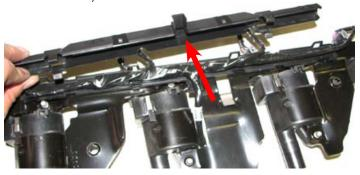
38. Remove the factory valley tray, by unplugging the oil pressure sensor and the Active Fuel Management (AFM) system (if applicable). Use a 27mm wrench to remove the oil pressure sensor from the valley tray. Unbolt the eleven (11) bolts securing the valley tray using a 13mm socket.
