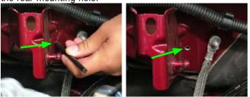
132. Secure the bracket to the firewall with the supplied sheet metal screw from the SUV hardware bag.
