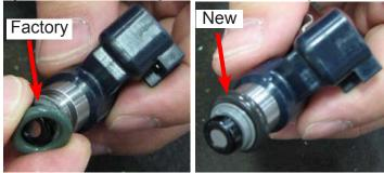
78. Remove and discard the factory installed metal clips on the injectors.
