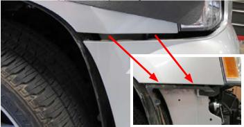
19. Using a 10mm socket, remove two (2) bolts from the bumper support brackets. One (1) from the driver side, the other from the passenger side. Unplug the fog lamps if equipped and carefully remove the fascia and set aside.
