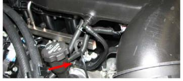
22. Using a 15mm socket and a breaker bar, remove the serpentine belt by rotating the tensioner clockwise until the belt can slide off the idler pulley.
