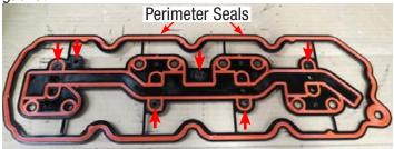
47. Using a 5/32" dill bit, drill out four (4) bleed holes in between the lifter bosses as shown. Place the gasket onto the supplied valley tray to verify that the drilled holes are aligned with the grooves on the valley tray. Clean the gasket to remove any debris and install onto the supplied valley tray. Proceed to Step 51.
