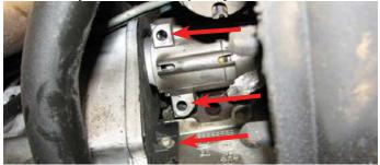
55. Install GM Flywheel Holding Tool #J-42386-A or equivalent, to prevent the crank from rotating while loosening the balancer bolt. Torque the bolts to 37 ft/lbs (51 Nm).
