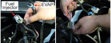
85. Re-connect all eight (8) fuel injector plugs. Reinstall the coil pack assemblies using a 10mm socket and the factory bolts. Then plug in the main coil pack harnesses and the coil pack boots.
