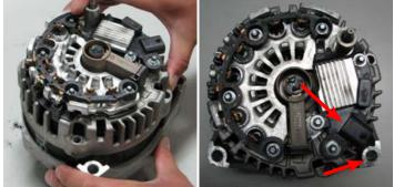
112. Using a 15mm socket and the supplied M10 x 90mm bolts in Bag #1, install the alternator onto the new alternator bracket and torque to 41 ft-lbs (55 Nm). Re-connect the alternator harness plug.
