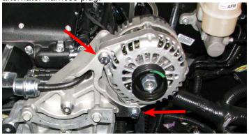
113. Remove factory alternator power cable and install supplied alternator power cable to factory location *(this may be on the firewall power junction or the positive battery terminal)*. Then route cable behind manifold and connect it to alternator using a 10mm socket.
