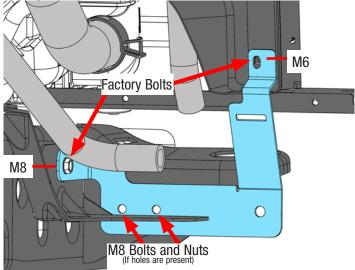
101. Secure the hose from the recovery tank to the inlet barb on the water pump with one (1) 3/4" hose clamp. Secure the hose from the LTR to the outlet barb on the water pump with one (1) 3/4" hose clamp. Making sure that the water pump outlet barb is pointing up, secure the water pump to the water pump bracket using the bracket strap and one (1) M8 x 30mm bolt from Bag #2.
