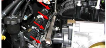
31. Remove the plastic cap on the schrader valve located on the passenger side fuel rail. Place a towel over the schrader valve and carefully release the pressure from the fuel system using a small flat head screwdriver or equivalent.
