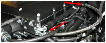
**NOTE:** Step 84 is performed to give additional slack to the right rear injector, EVAP and alternator connectors.
