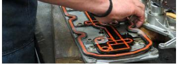
46. Using a precision grinding tool, grind down six (6) bosses on the gasket until they are flush with the gasket.
