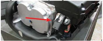
74. Remove protective tape from cylinder ports. Spray silicone lubricant or equivalent, onto the cylinder heads to help align the supercharger manifold.
