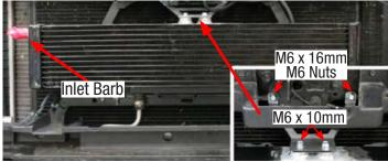
90. Mount lower LTR brackets to the lower LTR bungs using four (4) M6 x 35mm bolts and four (4) 1" spacers from the SUV hardware bag and Bag #2). Secure lower LTR brackets to the A-Frame with two (2) M6 x 16mm bolts from bag #2. Proceed to Step 78.
