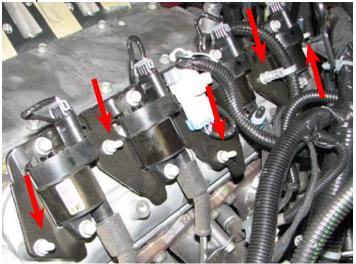
37. Using a small flat head screwdriver or equivalent, remove the plastic covers from the coil brackets (these will not be re-used).
