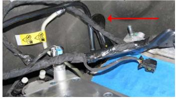
69. Two (2) of the stock intake manifold bolt holes in the cylinder heads break into the crankcase and are not used with this supercharger. Remove the tape covering the intake ports. Install two (2) button head bolts supplied in Bag #3 in the front passenger side and rear driver side intake manifold bolt holes.
