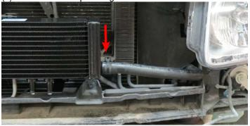
96. Install the Manifold to Recovery Tank hose onto the upper passenger side outlet barb on the manifold.
