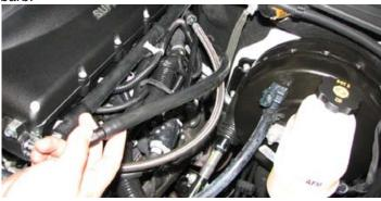
107. Install the rubber grommet from bag #1 into the hole located in the upper cavity of the alternator bracket. Using a 15mm socket, install the alternator bracket with the factory alternator bolts. Route the actuator hose through the grommet as shown, and re-connect to the actuator.
