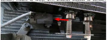
92. Using a hose clamp tool or equivalent, install the water pump to LTR hose to the LTR inlet barb with one (1) 3/4" hose clamp from Bag #2. Now route the hose around the radiator shroud and AC hard lines.
