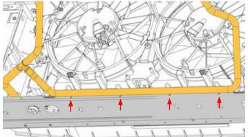
94. Install the other end of the LTR to Manifold hose onto the lower driver side manifold inlet barb.
