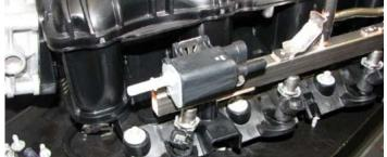
103. nstall the supplied EVAP bracket onto the driver side coil pack assembly stud using one (1) M6 nut from Bag #2. Stud location is in between the first and second coil packs. Install the factory EVAP on to the EVAP bracket as shown.
