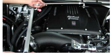
81. Lower the passenger fuel rail assembly onto the manifold lining up the injectors with their provisions on the manifold. Gently, push down on the rails until the injectors are fully seated. Secure fuel rail using a 5mm Hex tool and two (2) M6 x 12mm bolts from Bag #3.
