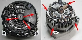
111. Clock the rear portion of the alternator clockwise one bolt position so that the harness plug points at the right mounting hole. Apply red Loctite to the bolt threads and reinstall the four (4) alternator bolts and plastic cover.
