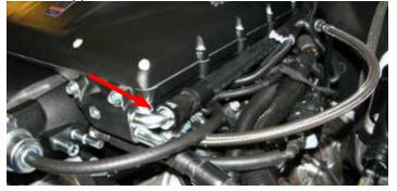
98. Using four (4) M6 x 16mm bolts from Bag #2, install the recovery tank bracket onto the recovery tank as shown.
