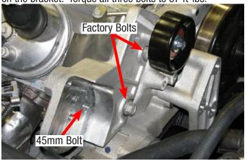
58. Apply blue loctite to the threads of one M8 X 20mm bolt supplied in Bag #1, then use a 12mm socket and the supplied washer to mount the pulley on the tensioner bracket and torque it to 18 ft-lbs.
