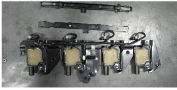
50. Tuck any loose wiring under each coil bracket then use a 10mm socket and the ten stock bolts to install the coil brackets on to each valve cover.
