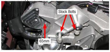
69. Apply blue Loctite to the threads of the M10 x 65mm socket head bolt supplied in Bag #1 then use an 8mm allen to install it in the left bolt hole provision of the tensioner bracket.
