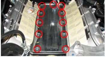
33. Use a small flathead screwdriver to remove the eight 0-rings from the stock valley plate and install them in the new valley plate. The oil baffle is not used.
