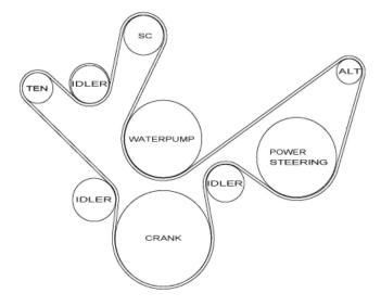
61. Use a breaker bar and a 16mm socket to push the tensioner enough to get the belt on. Double check the routing and make sure the belt is seated properly. Proceed to Step 78.
