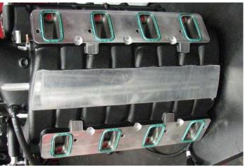
39. Clear the engine valley of any hoses, wires, tools, etc. and remove the tape covering the intake ports. With the assistance of one or more people, lift the supercharger assembly onto the engine.
