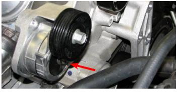
60. Route the serpentine belt (*not included*) according to the diagram below. Note that you must slide the belt around the bottom of the bracket to get the belt on the lower passenger side idler pulley.
