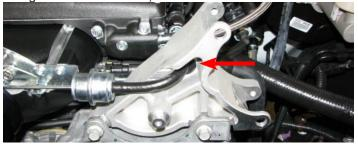
75. Remove the bolt, washer and bushing from the stock 90mm pulley and install them on the supplied 76mm pulley.
