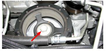
16. Install the drill guide and the M16 x 120mm guide bolt supplied in Bag #4 onto the end of the crankshaft.
