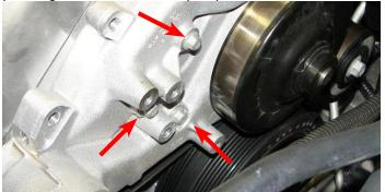
56. Using a 6mm Allen tool and the three 90mm bolts supplied in Bag #1, install the lower idler bracket onto the water pump then torque them to 18 ft-lbs.
