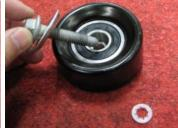
76. Apply Loctite to the threads on both idler pulley bolts. Then use a 15mm socket to install the 76mm idler pulley with the factory hardware to the left idler pulley location. Install the additional idler pulley to the right idler pulley location with the M8 x 20mm bolt and M8 washer from Bag #1. Verify that both pulleys spin freely.
