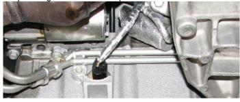
8. Use a 10mm socket to remove the starter support bracket bolt.
