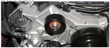
71. Apply blue Loctite to the threads of the M10 x 75mm Hex flange bolt supplied in Bag #1. Use a 15mm socket to install the supplied tensioner onto the tensioner bracket.
