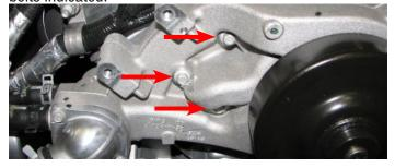
65. Apply blue Loctite to the threads of the M8 x 100mm bolts supplied in Bag #1 then use a 6mm Allen tool to install the idler bracket onto the water pump.
