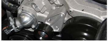
©2015 Edelbrock LLC Universal LS E-Force Supercharger 66. Use a 15mm socket to remove the nut retaining the ground strap on the passenger side cylinder head then use a 15mm deep socket to remove the ground strap stud.
