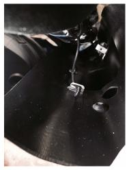
9. Pull the pillar away from the vehicle and install the tether. You will need to insert the first tab, twist the tether 45 degrees and insert the second tab.
