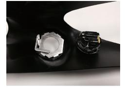
5. Remove speaker from factory pillar. Reinstall the speaker into the AutoMeter pillar mount, making sure the electrical connector points away from the "L" bracket.
