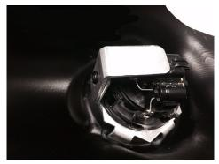
Position L bracket over speaker. While pressing down on the L bracket, tighten the Phillips head screw. Reconnect the wiring to the speaker.
