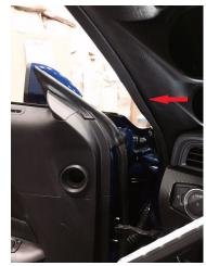
11. If a gap is present along the lower portion of your weather-stripping and the pillar, insert your fingers through the gauge opening and press the inside of the pillar outward to pop into place.
