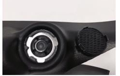
7. Align the tabs on the speaker cover with the cutouts in the A-pillar and snap into place.
