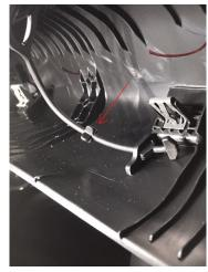
3. Release tether from factory pillar. You will need to slide both tabs on the tether through the slot by twisting the tether 45 degrees to align the last tab.
