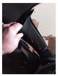
CAUTION: Please note the speaker is still connected. Do not pull the pillar all the way out at this step. Insert fingers behind factory pillar at top. Pull factory pillar away from the steel "A" pillar towards you while sitting in the driver's seat until clips have released. Then pull the pillar upward, towards the headliner, releasing the tail section from the dash area.
