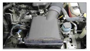
8. Release the four clips which secure the upper air box to the lower air box and then remove the intake tube and upper air box from the vehicle.
