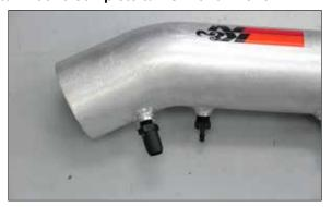
25. Install the 3/16 vent fitting into the K&N® intake tube as shown.
