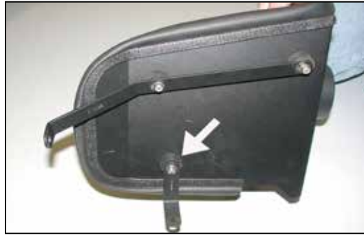
18. Install the "L" bracket onto the heat shield as shown, but do not tighten at this time.
