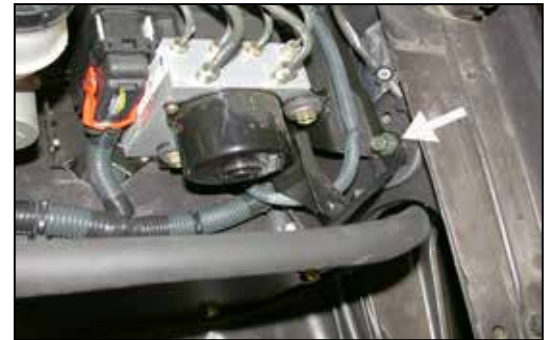
23. Using the bolt from step 12 secure the angle bracket to the ABS bracket as shown.
