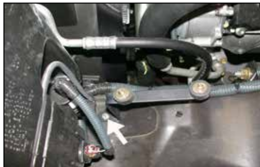
20. Install the "Z" bracket into the vehicle and secure it to the threaded hole from step 11 using the provided hardware as shown.
