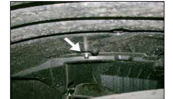
22. Secure the "L" bracket to the hole from step 10 on the inner fender panel with the provided hardware as shown.
