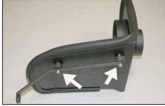
16. Install the angle bracket onto the heat shield and secure with the provided hardware but do not tighten at this time.
