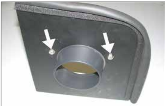
14. Using the provided tube of thread locker, apply two drops to the hex bolts and secure the filter adapter to the heat shield with the provided hex bolts and wave washers as shown.
