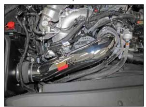
13. Install the K&N® intake tube into the coupler installed onto the filter adapter and then into the coupler installed onto the filter inlet. Adjust the tube for best fit and then secure with the provided hose clamps.
