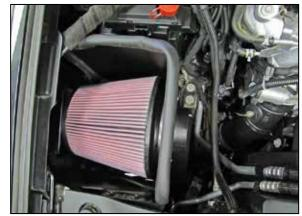
9. Flex the heat shield inward towards the engine then install the K&N® air filter onto the filter adapter and secure with the provided hose clamp. Secure the heat shield with two of the remaining factory bolts from step #5.
