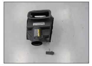
11. Remove the mass air sensor from the air filter housing.
