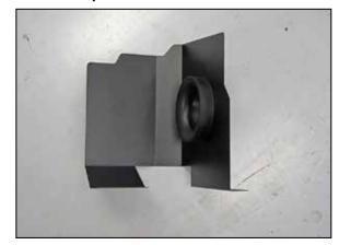
6. Install the provided filter adapter into the K&N® heat shield and secure with the provided hardware.
