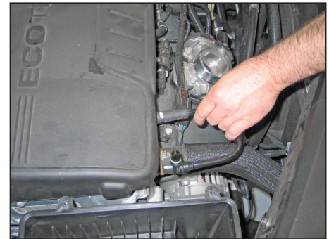
8. Remove the crankcase vent hose from the valve cover port.
