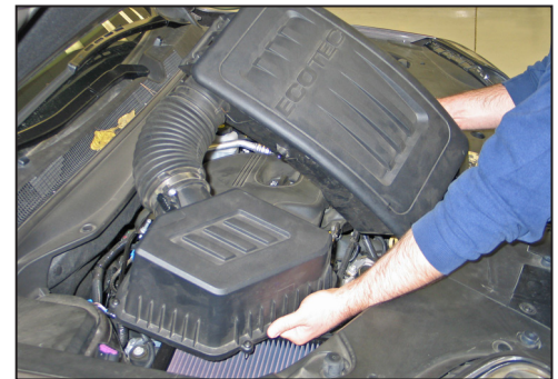
6. Remove the intake plenum and upper airbox from the vehicle.
