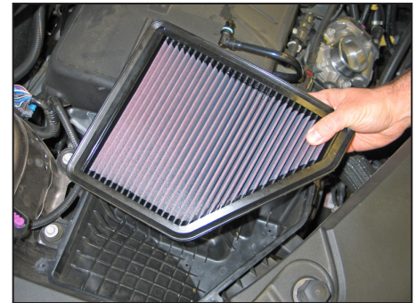
7. Remove the air filter from the lower airbox.
