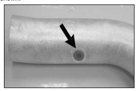
19. Install the provided rubber grommet into the hole on the  $K\&N^{\circledR}$  intake tube as shown.
