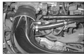
23. Install the provided 5/8" silicone hose onto the stock plastic crankcase vent line. Then, install the open end of the 5/8" ID silicone hose onto the K&N® intake tube and secure with the provided hose clamps.
