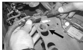
9. Unclip the mass air sensor wire harness from the air cleaner tray, then, disconnect the secondary mass air sensor electrical connection and remove the air cleaner assembly.
