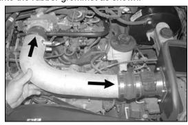
21. Slide the K&N<sup>®</sup> intake tube into the silicone hump hose, then, slide the silicone step hose onto the throttle body as shown.
