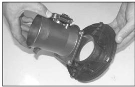
13. Remove the mass air sensor from the housing cover as shown.
