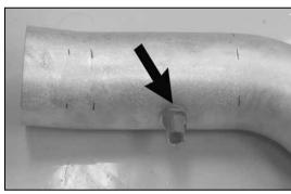
20. Install the air temperature sensor from step 8 into the rubber grommet as shown.
