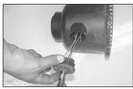
10. Disassemble the air cleaner assembly, then, pull the plastic wire cover and rubber boot back on the mass air electrical connection as shown.
