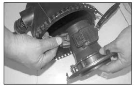
12. Disconnect the mass air sensor electrical connection as shown.
