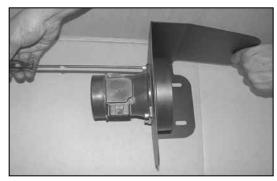
14. Bolt the stock mass air sensor onto the provided heat shield using the provided mass air adapter, gaskets and the provided hardware as shown.
