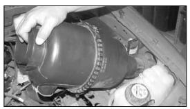
8. Pull firmly upwards to release the air cleaner assembly from the stock grommets located on the inner fender.
