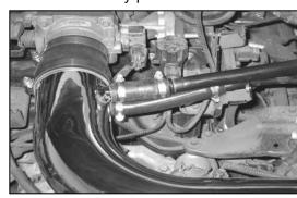
25. On V8-5.4L models slide the provided 5" long silicone hose onto the hard line, then trim hose for best fit before connecting to the vent on the K&N® intake tube as shown.
