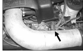
26. Reconnect the air temperature sensor electrical connection as shown.
