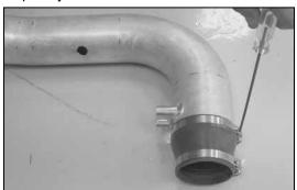
18. Install the provided silicone step hose and hose clamps onto the K&N<sup>®</sup> intake tube and tighten as shown.
