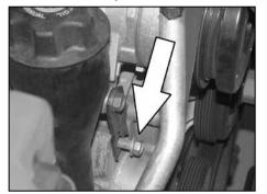
8. Remove the lower A/C bracket bolt shown with a 15mm socket.
