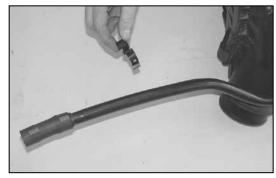
23. On 2005 and earlier vehicles remove the crankcase vent tube mounting clip from the crankcase vent tube on the airbox as shown.
