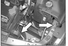
11. On 2008 and earlier models, remove the core support mounting bolt shown with a 13mm wrench, and pull out the stock airbox mounting grommet shown.
