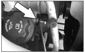
20. Line up the bracket with upper alternator mount and install the provided spacer, washer and hex bolt as shown.
