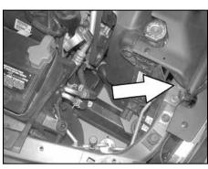
11a. On 2009 and later vehicles, the mounting bolt used has been eliminated. The heat shield bracket will need to move to the left mounting bolt which is under the radiator cover. It may be necessary to loosen the radiator cover.
