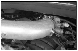
19. Slide the K&N $^{\odot}$  intake tube into the silicone hose on the throttle body as shown.
