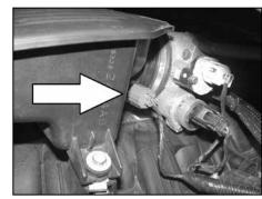
6. Depress the locking tab on the air temp sensor electrical connection and disconnect the air temp electrical connector.
