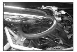
22a. On 2006 and later vehicles connect the crankcase vent hose installed in step #7c to the K&N<sup>®</sup> intake tube as shown.
