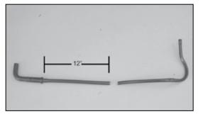
7b. On 2006 and later vehicles, measure 12" from the crankcase check valve and cut the crankcase vent tube as shown.
