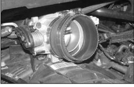
14. Install the silicone hose (084091) onto the throttle body and secure with the provided hose clamps.
