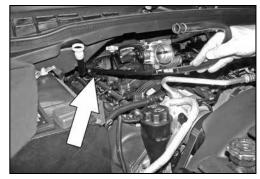
7a. On 2006 and later vehicles, disconnect the crankcase vent tube from the rear of the intake manifold.
