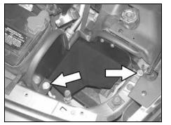
13. On the 2008 and earlier models install the K&N<sup>®</sup> heat shield assembly and secure the mounting bracket to the radiator core support with original bolt removed in step #11. Secure the rear of the heat shield to the 3/8" threaded insert with the provided hardware.
