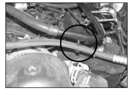
24. On 2005 and earlier vehicles install the crankcase vent tube mounting clip onto the A/C line and crankcase vent tube as shown.
