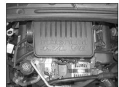
2. On 2005 and earlier vehicles, disconnect the crankcase vent tube from the vent hose junction above the alternator.
