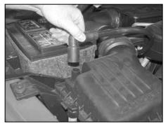
2a. On 2006 and later vehicles, disconnect the crankcase vent tube from the airbox lid as shown.
