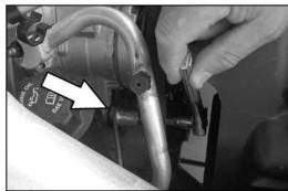
21. Snug the hex bolt but do not tighten completely at this time.
