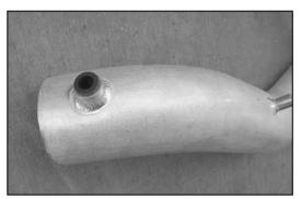
17. Install silicone hose into fitting on the  $K\&N^{\otimes}$  intake tube as shown.
