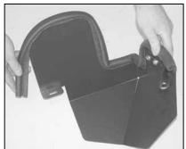
10. Install the provided edge trim onto the heat shield.
