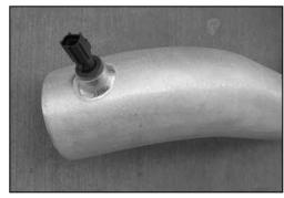
18. Install the air temperature sensor into the vent on the  $K\&N^{\otimes}$  intake tube as shown.
