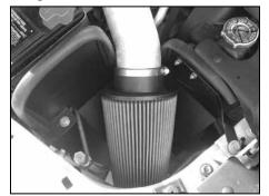
26. Install the K&N<sup>®</sup> air filter and secure with the provided hose clamp as shown.
