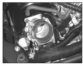
20. Install the supplied silicone hose (084014) onto the throttle body and secure it with the provided hose clamp.
