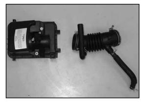
11. Loosen the hose clamp that secures the stock intake hose to the mass air sensor. Disconnect the intake hose from the mass air sensor as shown.
