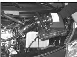
6. Release the two upper air box mounting clips and then remove the upper air box and intake tube assembly as shown.
