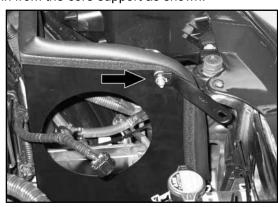
16. Attach the supplied heat shield bracket (06720) onto the heat shield as shown. Be sure to place one of the provided spacers between the heat shield and bracket.
