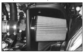
24. Install the K&N® Air Filter onto the mass air sensor and secure it with the provided hose clamp.
