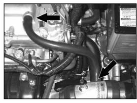
25. Install the supplied silicone hose onto the fitting on the valve cover. Attach the other end to the vent port on the K&N® intake tube.
