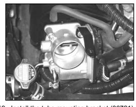
19. Install the tube mounting bracket (06721) onto the throttle body and secure it with the bolt removed in the previous step (Step 18).
