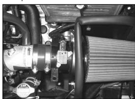
26. Reconnect the mass air sensor electrical connection and secure the mass air sensor wiring harness to the mass air sensor housing.
