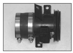
22. Install the remaining silicone hose (084014) onto the mass air sensor and secure it with the provided hose clamp.
