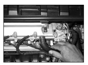
4. Release the spring clamp that secures the crank case vent hose to the valve cover. Then remove the crank case vent hose from the valve cover port as shown.
