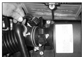
3. Depress the locking tab on the mass air sensor electrical connection and disconnect the electrical connector from the mass air sensor. Unhook the mass air sensor wiring harness from the mounting tabs on the air box.
