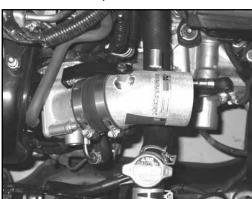
21. Install the K&N® intake tube into the silicone hose on the throttle body and align with the mounting bracket installed during step #19. Secure the intake tube with the provided hardware.
