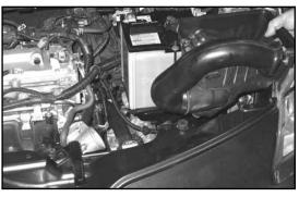
8. Release the mass air sensor wiring harness from the lower air box and then remove the lower air box from the vehicle as shown.
