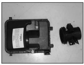
12. Remove the two bolts that secure the mass air sensor to the upper air box and then remove the mass air sensor as shown.
