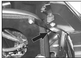
17. Attach the other end of the heat shield mounting bracket to the core support with the provided hardware. Be sure to place the remaining spacer between the bracket and under side of the core support.
