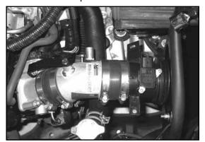
23. Pass the mass air sensor assembly through the heat shield and secure it to the intake tube with the provided hose clamp as shown.
