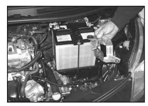
10. Unhook the mass air sensor wiring harness from the air box mounting bracket and then remove the air box mounting bracket from the vehicle.
