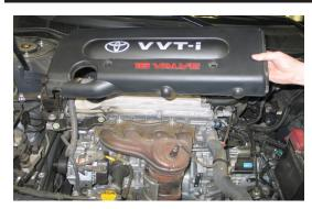
10. Remove the two nuts that secure the engine cover; then, remove the engine cover from the vehicle and set aside.
