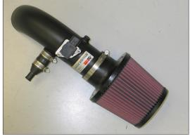
30. Install the air filter onto the intake tube secure using the provided hose clamp.
