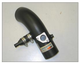
27. Install the stock crank case vent chamber into the silicone hose installed onto the intake tube secure with the provided hose clamp.
