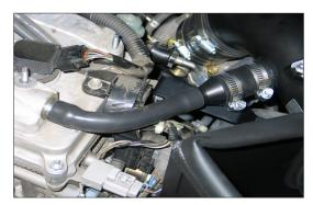
32. Install the provided crank case vent hose onto the crank case vent chamber and valve cover fitting.
