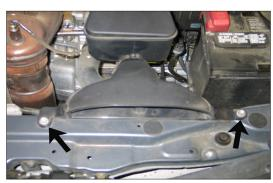
5. Remove the two bolts that secure the fresh air intake to the radiator core support. Note: These bolts will be re-used, do not
