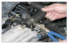
11. Using a pair of pliers, loosen the hose clamp that secures the crank case vent hose to the valve cover; then, disconnect the crank case vent hose from the valve cover.
