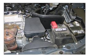
22. Install the fresh air intake onto the provision on the heat shield and adjust for proper fit; then, fasten with the stock bolts removed in step #5.
