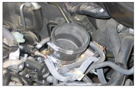
15. Install the provided silicone step hose (08095) onto the throttle body and secure with the provided hose clamp.
