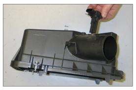
28. Remove the two screws that secure the mass air sensor to the air box. Remove the mass air sensor.
