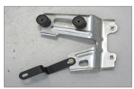
19. Install the supplied "Z" bracket (26655) onto the air box mounting bracket.
