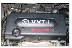
33. Install the stock engine cover and secure with the stock mounting bolts removed in step #10.
