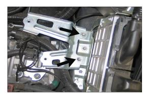
9. Remove the two bolts that secure the lower air box mounting bracket to the inner fender and set aside; then, remove the mounting bracket from the vehicle.
