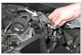
23. Secure the supplied "L" bracket (070066) to the pulse width modulated (PWM) switching valve using the stock screw removed in step #13.
