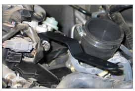
16. Install the intake tube mounting bracket (26654) onto the engine using the provided hardware.
