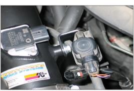
34. Secure the "L" bracket and pulse width modulated (PWM) switching valve assembly to the intake tube using the provided hardware.
