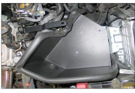
21. Place the heat shield into position and secure the air box mounting bracket to its original location using the two stock bolts removed in step #9.
