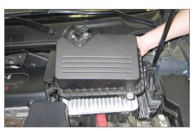
4. Remove the air box lid from the vehicle.
