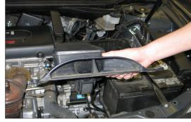
6. Remove the fresh air intake from the lower air box; then, remove from the vehicle.
