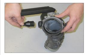
25. Release the clamp; then remove the crank case vent hose chamber from the stock intake tube.
