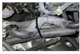
14. Using the provided tie-wrap, secure the heater hoses to the throttle body bypass hoses as shown in the photograph.
