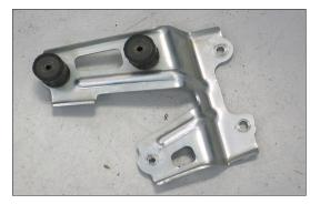
18. Install the two rubber mounted studs onto the air box mounting bracket as shown.
