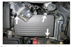
3. Loosen the stock intake tube hose clamp and two upper air box mounting bolts as shown in the photograph.
