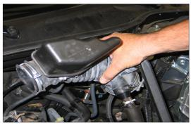
12. Using a pair of pliers, loosen the hose clamp that secure the stock intake tube to the throttle body; then, remove the intake tube from the throttle body as shown in the photograph.
