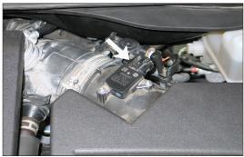
2. Disconnect the mass air sensor electrical connection and release the wiring harness from the air box lid.
