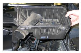
8. Remove the lower air box from the vehicle as shown in the photograph.
