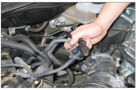
13. Position the intake tube in a fashion that will allow access to the Pulse width modulated (PWM) switching valve mounting screw; then remove the screw. Remove the entire intake tube assembly from the vehicle.
