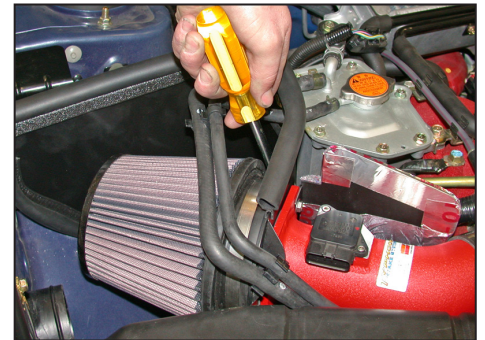
29. Install the K&N® air filter and and secure with the provided hose clamp as shown.
