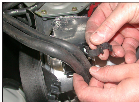
22. Remove the coolant hose clip as shown.
