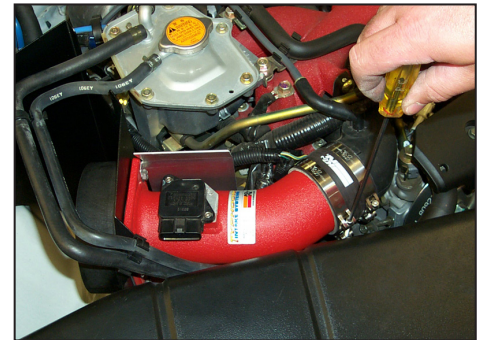
27. Tighten the hose clamp at the silicone hose as shown.
