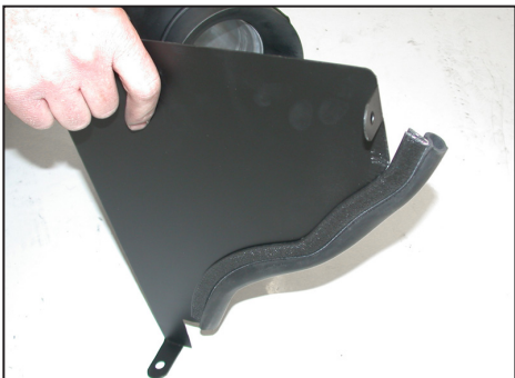
16. Install the provided edge trim onto the heat shield and trim as shown.
