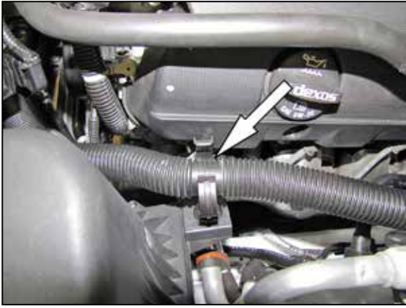
7. Open the clamp securing the sound tube to the air filter housing.
