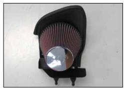
12. Install the K&N<sup>®</sup> air filter onto the filter adapter and secure with the provided hose clamp.
