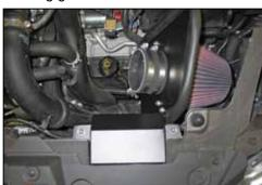
14. Install the provided fresh air scoop onto the core support and then secure the scoop to the core support and heat shield with the provided bardware
