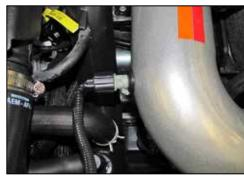
19. Reconnect the inlet air temperature sensor electrical connection.
