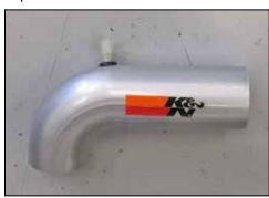
17. Install the provided grommet and the inlet air temperature sensor into the K&N® intake tube as shown.
