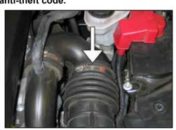
2. Loosen the hose clamp shown that secures the factory intake tube.
