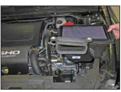
7. Lift up the airbox and remove it from the vehicle.
