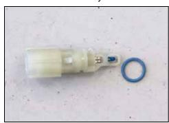
16a. Remove the grommet from the inlet air temperature sensor as shown.
