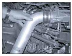
24. Install the complete K&N® intake assembly into the vehicle and slide the tube into the silicone hose on the throttle body as shown.
