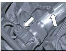
27. Reconnect mass air sensor electrical connection and insert the air temp sensor into the grommet as shown.
