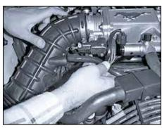
7. Detach the PCV line from the intake tube.
