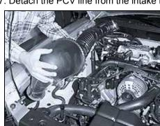
8. Remove the entire air intake assembly.
