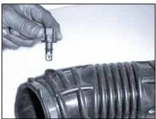
10. Remove the air temp. sensor from stock intake tube as shown.
