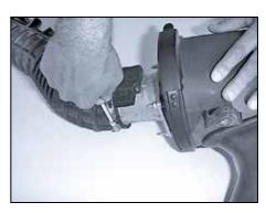
9. Loosen the hose clamp and detach the intake tube from the mass air sensor.
