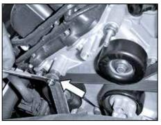
13. Loosen and remove the nut from the protruding stud on the engine.
