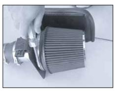
23. Install the K&N® air filter onto the filter adapter and secure with the provided hose clamp as shown.
