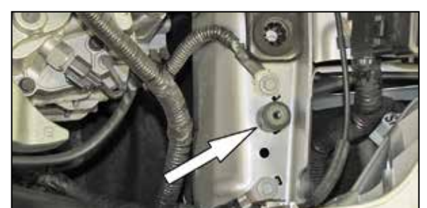
7. Install the provided rubber mounted stud into the inner fender as shown. NOTE: If this hole is not threaded, remove the self tapping bolt from the ground wire and use it to tap threads in this hole first. Be sure to reattach the bolt to the ground wire.
