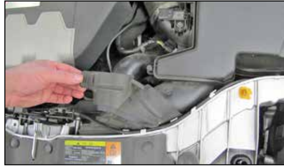
3. Disconnect the fresh air inlet boot.
