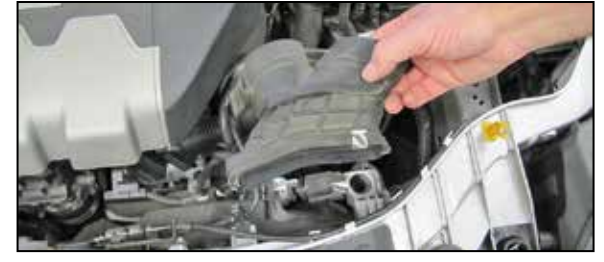
6. Remove the fresh air duct from the core support as shown.
