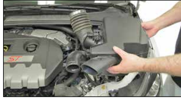
5. Remove the air box from the engine compartment. NOTE: K&N Engineering, Inc., recommends that customers do not discard factory air intake.
