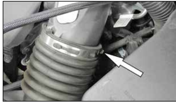
4. Loosen the hose clamp securing the intake hose to the plenum.
