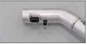
15. Install the mass air sensor into the  $K\&N^{\otimes}$  intake tube and secure with the provided hardware.
