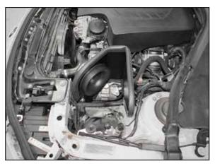
12. Set the heat shield into position so the mounting stud engages with the factory air filter housing mounting grommet and aligns with the fresh air intake duct, secure the fresh air intake duct with the provided hardware but do not completely tighten at this time.
