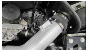
17. Connect the crank case vent hose to the fitting installed into the K&N<sup>®</sup> intake tube and reconnect the mass air sensor electrical connection.
