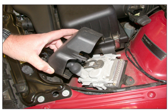
3. Unclip and remove the high intensity discharge unit cover as shown.
