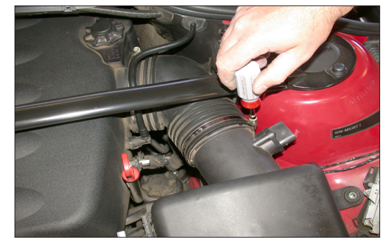
8. Loosen the hose clamp on the air cleaner flange as shown.
