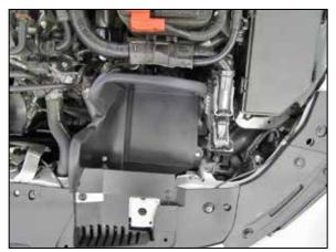
8. Install the heat shield assembly into the vehicle and secure with the provided hardware and one of the push pins that originally secured the fresh air intake. Install the three remaining push pins to fill the original mounting holes.
