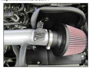
15. Route the mass air sensor wiring harness through the hole provided in the heat shield and then reconnect the mass air sensor electrical connection.
