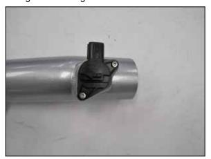
9. Remove the mass air sensor from the factory intake tube and install it into the K&N® intake tube and secure with the provided hardware.
