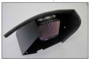
9. Install the K&N® air filter onto the filter adapter and secure with the provided hose clamp.
