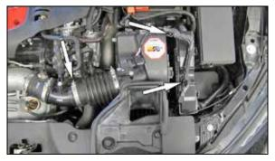
3. Release the upper air filter housing clips and loosen the hose clamp that secures the intake hose to the turbo inlet pipe. Remove the upper air filter housing and intake tube from the vehicle.
