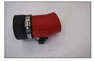
12. Install the provided coupler (084091) onto the inlet side of the K&N $^{\odot}$  intake tube and secure with the provided hose clamp.
