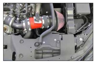
16. Install the provided fresh air duct and secure with the provided hardware. Install the remaining length of edge trim onto the fresh air duct.
