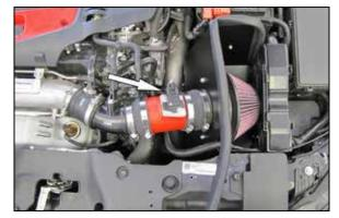
15. Remove the plastic harness holder from the mass air sensor harness. Install the provided split harness cover and secure with electrical tape. Route the harness through the notch in the front of the heat shield and then reconnect the mass air sensor electrical connection.
