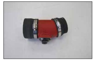
13. Install the provided coupler (084034) onto the outlet side of the K&N<sup>®</sup> intake tube and secure with the provided hose clamp.
