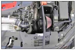
10. Set the heat shield assembly into position on the rubber mounted studs and then secure with the provided hardware.
