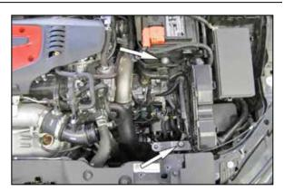
5. Install the two provided rubber mounted studs into the factory air filter housing mounting locations as shown.
