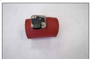
11. Remove the mass air sensor from the factory housing and install it into the K&N<sup>®</sup> intake tube as shown.
