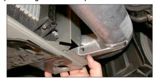
40. Secure the bracket to the core support using the provided hardware.
