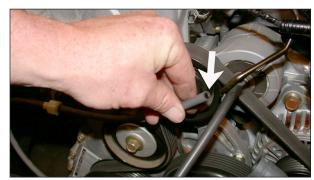
22. Disconnect the vacuum hose from the hard line as shown.
