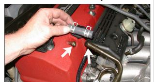
11. Remove the stock rubber hose from the crank case vent on the cam cover and from the hard line as shown.
