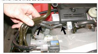
16. Using the remaining piece of 4mm hose from step 15, trim a 2-1/2" length of hose and reconnect the upper hard lines as shown.
