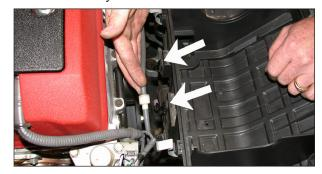
8. Unclip the vacuum hose from the rear of the lower air cleaner assembly as shown.
