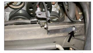
25. Using the provided hardware secure the "Z" bracket to the original air cleaner mounting location as shown.
