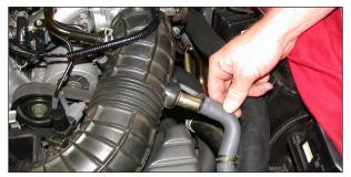
3. Remove the air injection pump hose from the stock intake tube as shown.
