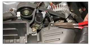
7. Unclip the wire harness from the lower air cleaner assembly as shown.
