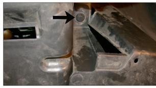
36. Remove the two remaining push clips located on both sides of the inner wheel house as shown.
