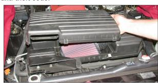
2. Unclip the six over center clamps, then, remove the air cleaner lid as shown.
