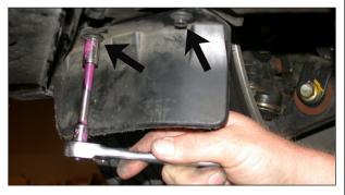
33. Raise the vehicle up and support it with jack stands, then, remove the rock guard from the lower right side valance located in front of the front tire as shown.
