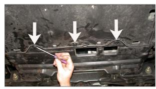
35. Remove the 5 push clips that secure the underbody splash guard as shown.
