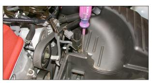
6. Remove the solenoid from the lower air cleaner assembly as shown.
