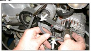
18. Disconnect the vacuum hose from the upper solenoid port and from the hard line as shown.
