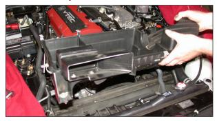
10. Remove the lower air cleaner assembly as shown.
