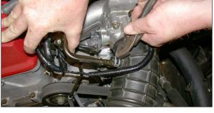
4. Remove the crank case vent hose from the stock intake tube as shown.
