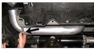
39. Slide the K&N<sup>®</sup> cold air tube into the silicone hose, then, line up the bracket with the radiator core support as shown.
