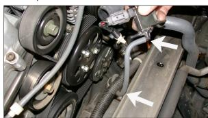
20. Reroute the vacuum hose behind the wire harness, then, reconnect the vacuum hose to the lower solenoid port as shown.
