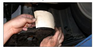
38. Using the provided template, use a white paint pen and mark the trim lines on the inner fender valance, then cut with an appropriate air or hand tool
