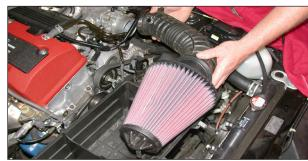
5. Loosen the hose clamp at the throttle body, then remove the intake tube and filter as shown.
