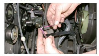
24. Using the provided hardware secure the solenoid to the provided "Z" bracket as shown.
