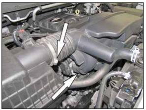
2. Loosen the two hose clamps that secure the intake plenum to the throttle body and air filter housing.
