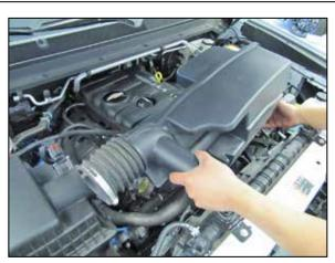
5. Remove the intake plenum from the vehicle.
