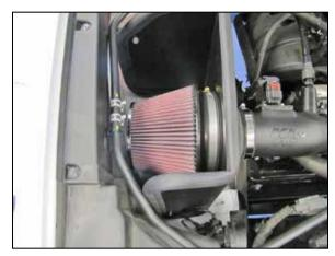
24. Install the K&N® air filter and secure with the provided hose clamp.
