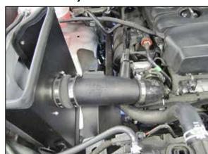
21. Install the Intake tube assembly into the coupling hose at the filter adapter and then connect it to the throttle body, adjust the tube and hoses for best fit and then secure with the provided hose clamps.
