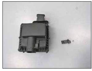
16. Remove the two screws securing the mass air sensor and then remove the mass air sensor from the factory air filter housing.
