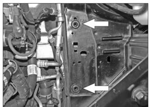
13. Remove the two mounting grommets shown from the inner fender.
