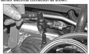
3. Release the locking tab and disconnect the crank case vent tube as shown.
