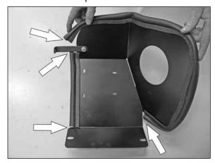
29. Install the provided edge trim onto the heat shield as shown.
