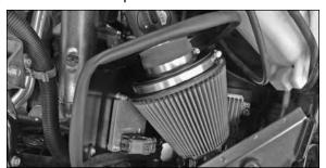
38. Install the air filter assembly onto the mass air sensor and secure with the provided hose clamp.
