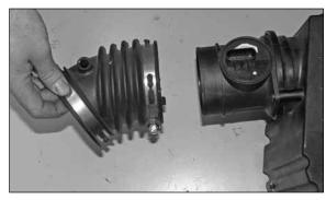
21. Loosen the hose clamp, which secures the stock intake tube to the mass air sensor, and then remove the hose from the sensor as shown.
