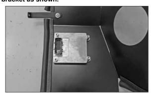
30. Secure the transmission control module to the heat shield with the provided hardware as shown. NOTE: Four washers should be placed between the heat shield and module to form an air gap.
