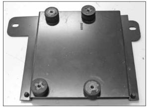
15. Install the four rubber mounted studs onto the engine control module mounting bracket as shown using the provided hardware.
