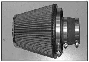
37. Install the silicone hose (08051) onto the K&N<sup>®</sup> filter assembly as shown and secure with the provided hose clamp.
