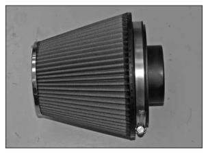
36. Install the filter adapter into the K&N® air filter as shown and secure with the provided hardware.
