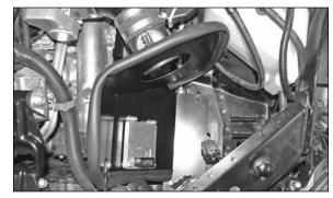
33. Install the heat shield assembly onto the inner fender and secure the mounting bracket to the radiator mount using the factory bolt removed in step #32.
