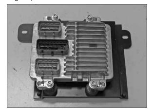
16. Install the engine control module onto the mounting bracket as shown with the provided hardware.
