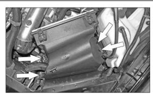
7. Depress the four air box housing retaining clips shown.
