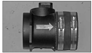
26. Install the silicone hose (08690) onto the mass air sensor as shown and secure with the provided hose clamps.
