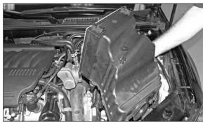
8. Remove the upper air box housing from the vehicle as shown.
