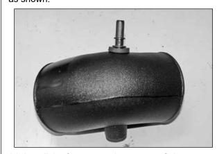
24. Install the factory crank case vent fitting removed in step #20 into the grommet installed into the K&N® intake tube in step #19.
