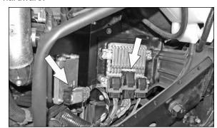
35. Reconnect the engine control module and transmission control module electrical connections.
