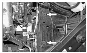
31. Install the two inserted nuts into the air box mounting grommet holes as shown.
