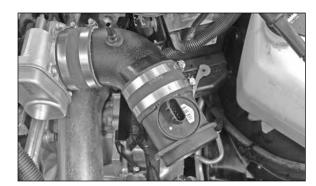
27. Install the mass air sensor assembly onto the K&N® intake tube as shown and secure with the provided hose clamp.
