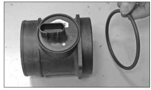
23. Remove the "O" ring from the mass air sensor as shown.
