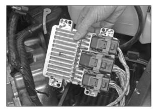
10. Release the engine control module from the mounting clip and lift the module from the base as shown.
