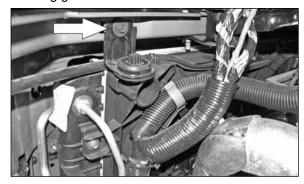
32. Remove the top left radiator mounting bracket bolt shown.
