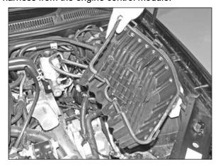
12. Pull up the lower air box housing to release it from the mounting grommets and then remove the housing from the vehicle as shown.
