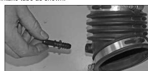
20. Remove the crank case vent fitting from the stock intake tube as shown.
