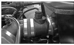
41. Reconnect the mass air sensor electrical connection.
