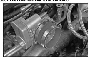
18. Install the silicone hose (08690) onto the throttle body and secure with the provided hose clamp.
