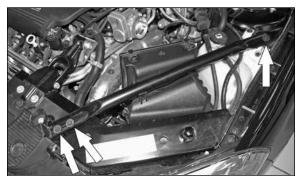
6. Remove the three body support brace mounting bolts shown and then remove the support brace from the engine compartment.
