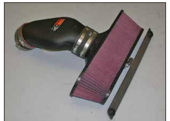
10. Install the air filter mounting bracket onto the air filter as shown and secure with the provided hardware.
