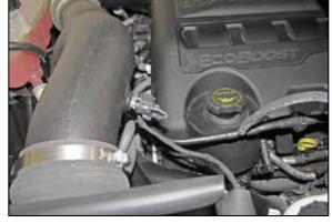
18. Reconnect the inlet air temperature sensor electrical connection using the provided extension harness.
