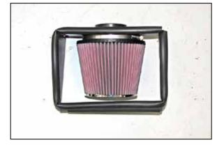
10. Install the K&N<sup>®</sup> air filter onto the filter adapter and secure with the provided hose clamp.
