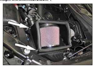
12. Install the heat shield/filter assembly onto the lower air filter housing and secure with the factory retaining clips.
