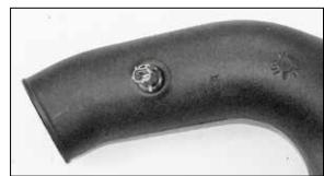
18. Remove the O-Ring from the inlet air temperature sensor and then install it into the grommet installed into the K&N® intake tube. .
