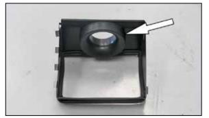
10. Install the provided filter adapter into the heat shield and secure with the provided hardware.
