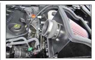
13. Install the provided coupling hose (08699) onto the filter adapter and secure with the provided hose
