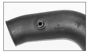
16. Install the provided grommet into the K&N® intake tube as shown.
