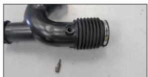
17. Unlock the inlet air temperature sensor and rotate it counter clockwise, remove the sensor from the factory air filter housing.
