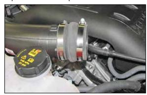
15. Install the provided coupling hose (087121) onto the passenger side turbo inlet tube and secure with the provided hose clamp.
