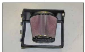
11. Install the K&N® air filter onto the filter adapter and secure with the provided hose clamp. NOTE: Drycharger® air filter wrap; part # RC-5173DK is available to purchase separately. To learn more about Drycharger® filter wraps or look up color availability please visit http://www.knfilters.com®.
