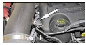
20. Reconnect the inlet air temperature sensor electrical connection.
