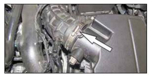
4. Loosen the hose clamp securing the factory intake tube to the air box housing.
