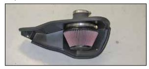
15. Install the K&N $^{\circ}$  air filter onto the filter adapter and secure with the provided hose clamp.
