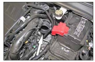
8. Install the provided hump hose (087121) onto the turbo inlet and secure with the provided hose clamp.
