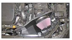
16. Set the heat shield assembly into the vehicle. The mounting stud will insert into the factory air box mounting grommet and the front of the heat shield will be secured to the core support with the provided hardware.
