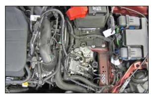
9. On 2008 and later model vehicles with the pressure sensor, connect the provided Inlet air temperature sensor extension harness to the open connector for the sensor. Then route the wiring harness along the hoses and reconnect the pressure sensor electrical connection.
