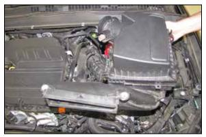
6. Lift up the air box to dislodge it from the mounting grommets and then remove it from the vehicle.
