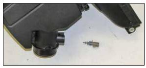
19. Remove the inlet air temperature sensor from the factory air box and remove the O-Ring from the sensor.
