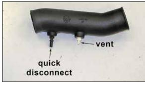
18. Install the provided 1/4"npt fittings into the K&N<sup>®</sup> intake tube as shown.
