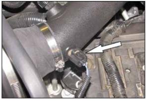
23. Using the provided extension harness, connect the inlet air temperature sensor electrical connection.
