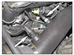
22. Connect the factory solenoid vent hose and the factory crank case vent hose to the fittings installed into the K $\&N^{\otimes}$  intake tube.
