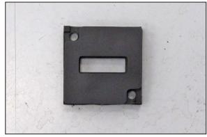
16. Install the provided gasket onto the K&N® mass air sensor adapter.
