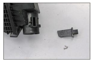
17. Remove the mass air sensor from the factory air box.
