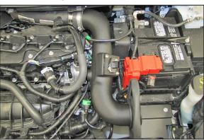
21. Install the K&N® intake tube assembly into the silicone hose at the turbo inlet pipe and then into the heat shield, adjust the tube for proper fit and then secure with the provided hose clamps.
