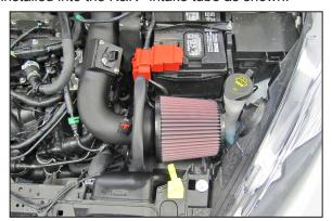
24. Install the K&N® air filter onto the intake tube and secure with the provided hose clamp. NOTE: Drycharger® air filter wrap; part # RX-4990DK is available to purchase separately. To learn more about Drycharger® filter wraps or look up color availability please visit http://www.knfilters.com®.
