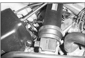
34. On models equipped with an external air temperature sensor, insert the air temp. sensor into the grommet on the intake tube.
