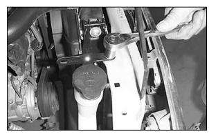
19. Attach the twist bracket to the front airbox mounting point on the radiator core support using the hardware provided.
