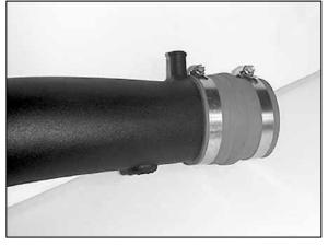
24. Install the silicone hose onto the  $K\&N^{\mbox{\scriptsize 0}}$  intake tube.
