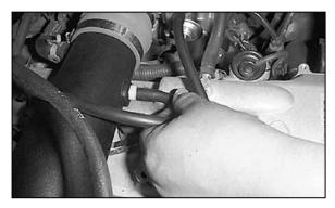
31. On models equipped with an A/C idle up magnetic valve vacuum line, attach the 1/4"id vent hose to the 1/8" barbed vent.
