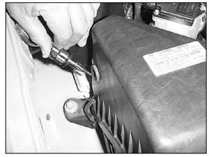
2. Remove the air temperature sensor from the airbox.
