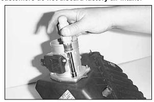
14. Loosen the 4 nuts and remove the mass air sensor from the airbox.
