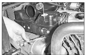
10. Loosen and remove the 2 nuts that retain the resonator assembly.
