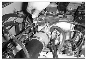
28. Tighten the hose clamps on the silicone hose.
