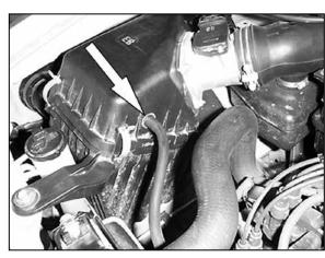
5. Disconnect the evaporative canister vent line from the airbox.
