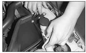
21. Install the heat shield assembly and secure to the brackets using the hardware provided.
