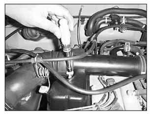
7. Loosen the hose clamp on the intake hose at the intake tube.
