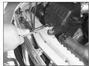
4. Loosen and remove the 3 bolts that retain the airbox.
