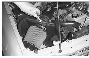
36. Install the air filter element and tighten the hose clamp.
