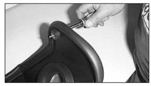
18. Attach the rubber mounted stud to the heat shield using the hardware provided.
