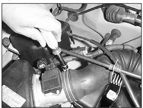
6. Loosen the hose clamp on the intake hose at the mass air sensor.
