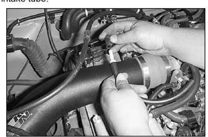
30. On models equipped with an A/C idle up magnetic valve vacuum line, connect the vacuum hose disconnected in step 11 to the 1/4"id vent hose using the 1/4" hose mender provided. (Items T and Y in exploded diagram).
