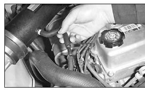
32. On models equipped with an evaporative canister vent line, connect the vent hose disconnected in step 5 to the 3/8"id vent hose using 3/8" hose mender provided. (Items U and Z in exploded diagram)
