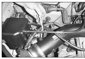
37. Secure the wiring harness to the throttle cable using the cable tie provided.
