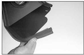
16. Install the trim seal onto the heat shield.
