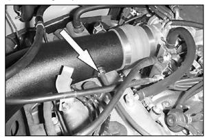
33. On models equipped with a fuel pressure regulator vacuum line attach the vacuum line to the 1/8" barbed vent.
