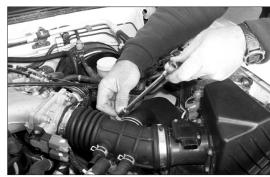
7. Loosen clamp on the resonator tube using a 10mm socket.
