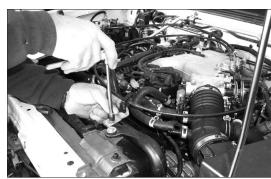
6. Disconnect the throttle cable bracket using a 10mm socket.
