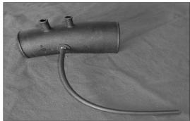
34. Install the the provided grommet and 4mm hose onto the intake tube as shown.
