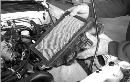
14. Remove the lower air filter housing as shown.
