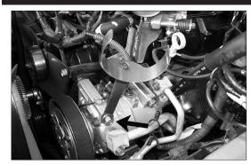
30. Install the saddle bracket assembly onto the AC compressor using the bolt that was removed in the previous step.
