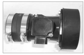
33. Install the silicone hose and the filter adapter onto the mass air sensor with the provided hardware.
