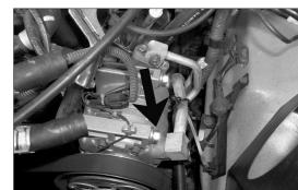
29. Remove the AC compressor mounting bolt.
