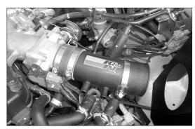
35. Install the K&N® intake tube onto the throttle body and secure the saddle bracket to the intake tube with the provided hose clamps.
