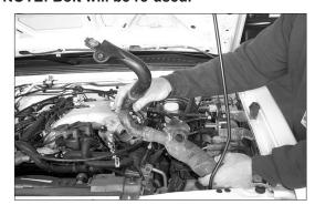
17. Remove the front resonator assembly as shown.
