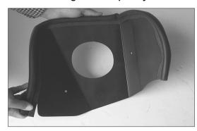
24. Install edge trim onto heat shield as shown. Trim if needed.
