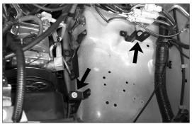
23. Install the two "L" brackets onto the vehicle as shown using the provided hardware.
