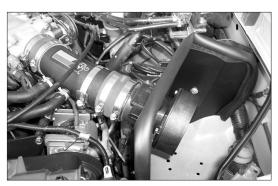
39. Install the mass air assembly onto the intake tube.
