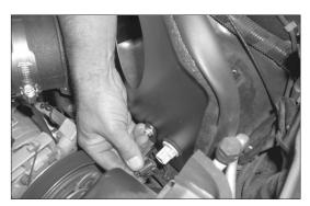
38. Reconnect the air temp sensor electrical connection as shown.
