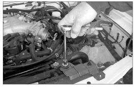
16. Remove bolt from front of resonator using a 10mm socket.
