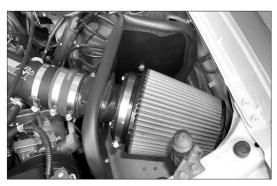
40. Install the K&N® air filter onto the intake tube.
