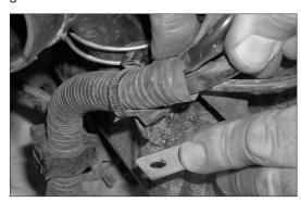
19. Using pliers, remove the wire loom clip.
