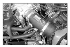
37. Reconnect the two vent lines to the intake tube.
