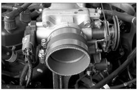
32. Install the silicone hose onto the throttle body with the provided hose clamp.
