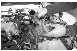
20. Remove the resonator box as shown.
