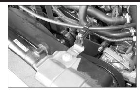
42. Re-install the throttle cable bracket using the provided nut and bolt.
