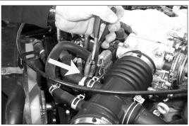
4. Squeeze the two hose clamps and slide back using pliers.
