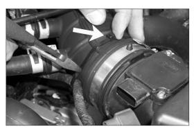
3. Lift up on the release tab to remove the factory zip-tie, as this will be reused in a later step.
