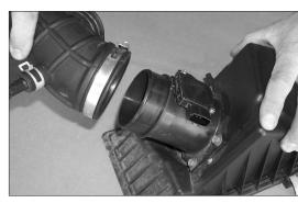
21 Loosen hose clamp using an 10mm socket and remove air duct tube from mass air sensor.
