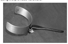
28. Install the saddle bracket onto the "L" bracket as shown.
