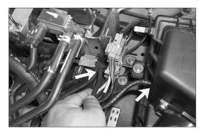
9. Remove vacuum line from bypass solenoid as shown.
