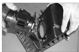
22. Remove the four bolts from mass air sensor housing using a 10mm socket and detach from airbox.
