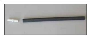
23. Assemble the silicone hose and hose mender as shown.
