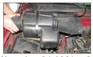
4. Loosen and remove the two bolts that secure the air inlet/resonator, then remove the assembly as shown.
