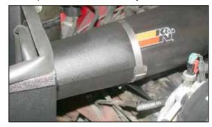
21. Secure the K&N® intake tube to the saddle bracket assembly with the provided hose clamp.
