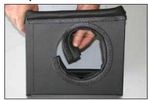
13. Install the short piece of trim seal to the heat shield as shown.
