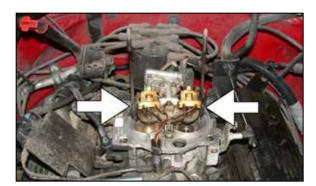
7a. On 92-95 vehicles, remove the two factory throttle body studs as shown.
