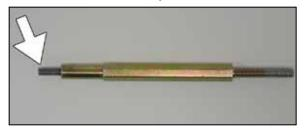
8a. Apply two drops of the provided thread locker onto the threads of the 5mm stud and then thread the stud into the tube mounting stud as shown.
