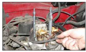
18. Remove the paper backing from the provided gasket and install the gasket onto the throttle body sticky side down.
