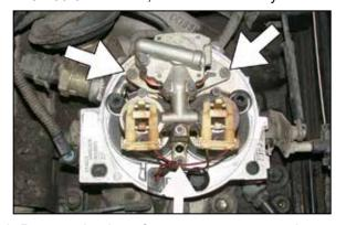
8. Remove the three factory torx screws as shown.
