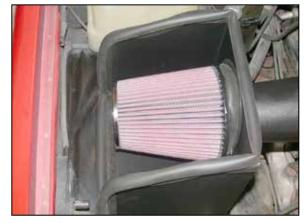
22. Install the K&N® air filter onto the K&N® intake tube as shown.
