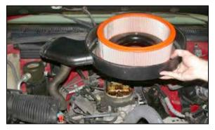
3. Disconnect the cold inlet tube and then remove the air cleaner base assebmly as shown.
