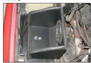
14. Install the heat shield to the inner fender using the provided hardware as shown.
