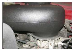
19. Install the  $K\&N^{\otimes}$  intake tube onto the throttle body.
