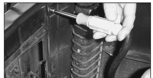
12. Remove the upper hex bolt from the plastic radiator valence.
