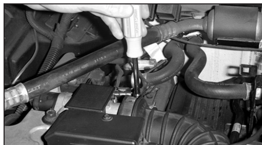
6. Loosen the hose clamp at the throttle body.
