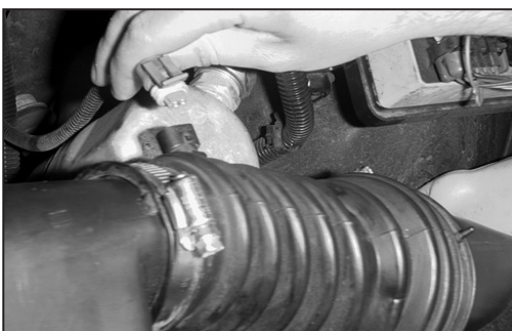
2. Disconnect the vehicle's air temperature sensor.
