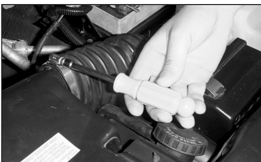
3. Loosen the hose clamp at the air intake plenum.
