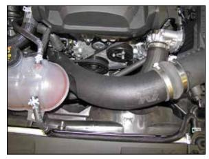
8. Install the provided hump coupler (08683) onto the K&N® intake tube, Install the intake tube into the coupler on the turbo and align the coupler with the air filter housing. Position the coupler onto the air filter housing and adjust the assembly for best fit. Secure the tube and couplers with the provided hose clamps.
