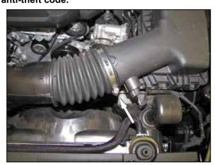
2. Loosen the hose clamp that secures the factory intake tube to the air filter housing.
