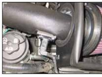
26. Re-connect the mass air sensor electrical connection as shown.
