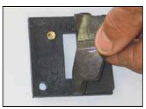
11. Install the provided gasket onto the mass air adapter as shown with the sticky side down.
