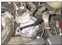
20. Install the tube bracket assembly onto the timing cover stud at the front of the engine as shown.
