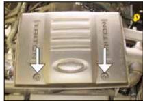
3. Remove the two bolts that secure the engine cover
