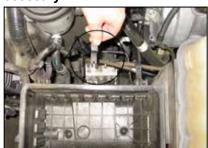
17. Remove the center latch from the lower air box as shown.
