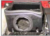
18. Install the heat shield and secure with the two remaining latches as shown.
