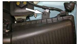
9. Remove the air box retaining bolt shown.
