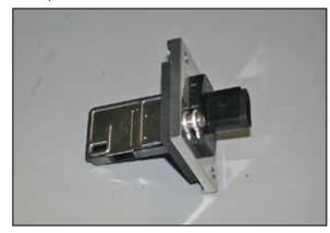
21. Using the screws removed in step #19, install the mass air sensor into the K&N® mass air adapter.
