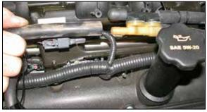
5. Disconnect the evaporative hose from the evaporative valve and cut the two tie wraps securing the hose to the bracket.
