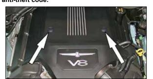
2. Remove the two plastic screws shown securing the engine cover.
