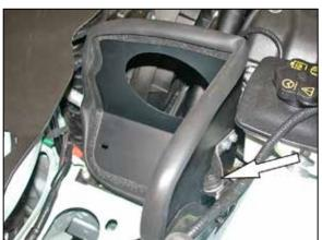
13. Install the heat shield into the vehicle and secure the bracket installed in step #12 to the factory air box mount with the factory bolt removed in step #0
