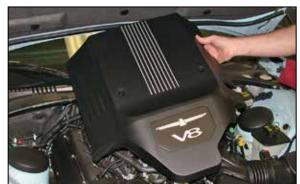
3. Pull up on the rear of the engine cover to dislodge from the retaining mounts, and then remove the engine cover from the engine.
