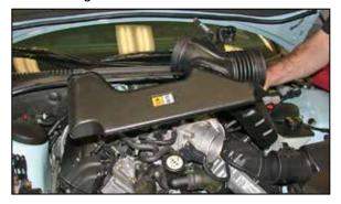
8. Remove the stock intake tube assembly from the vehicle.
