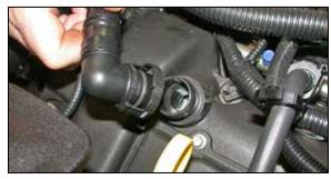
6. Depress the locking ring on the crank case vent hose, and then remove the crank case vent hose from the valve cover.
